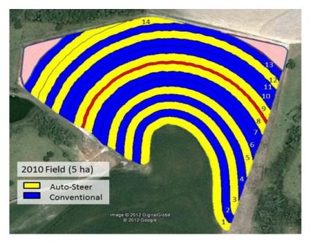
**Figure 3.** Experimental design used in 2011. Each replicate (colored strip) = 12 rows of peanuts or three 4-row passes. Numbers indicate strips used during data analysis.
