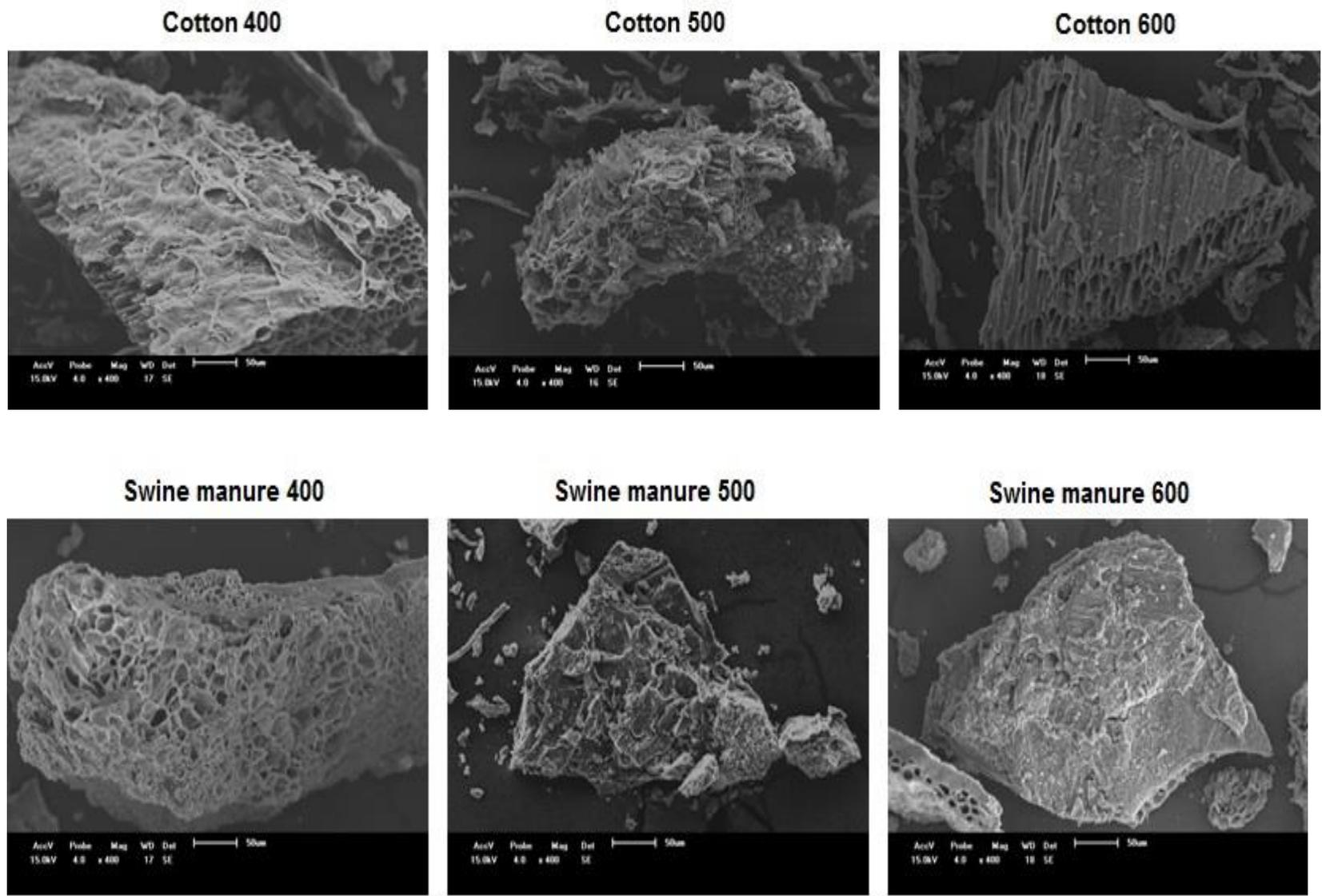
**Figure S4.** SEM images of cotton and swine manure biochars at 400, 500, and 600°C at x400 magnification (Shimadzu SSX-550 Superscan microscope).
