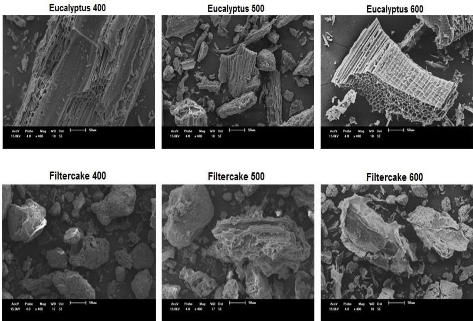
**Figure S5.** SEM images of eucalyptus and filtercake biochars at 400, 500, and 600°C at x400 magnification (Shimadzu SSX-550 Superscan microscope).
