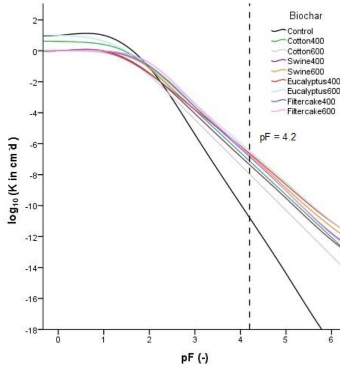
**Figure S7.** Hydraulic conductivity curves for packed biochar-soil mixtures, low and high temperatures of pyrolysis (HYPROP data;  $n=1$ ). pF 4.2 is the permanent wilting point.
