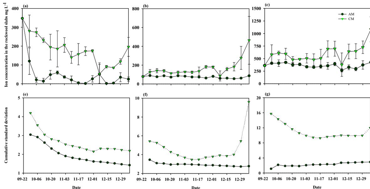
**Figure 8.** Changes in nutrient concentrations (mean  $\pm$  SD) of  $K^+$  (a),  $Mg^{2+}$  (b), and  $Ca^{2+}$  (c) and changes in cumulative standard deviation of nutrient concentrations of  $K^+$  (e),  $Mg^{2+}$  (f), and  $Ca^{2+}$  (g) in the rockwool substrates using the conventional (CM) and alternative (AM) nutrient-replenishment methods, respectively.
