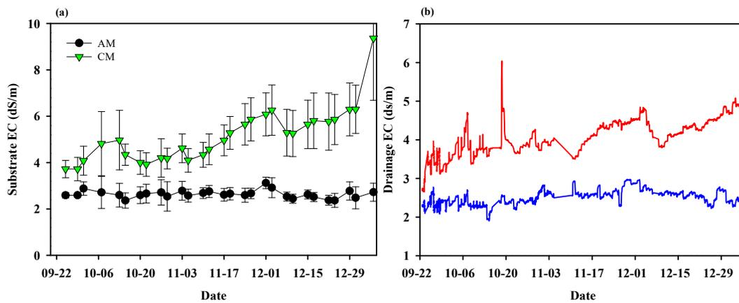
**Figure 4.** Comparison of electrical conductivity (mean  $\pm$  SD) in the rockwool substrate (a) and the drainage (b) of the closed-loop soilless culture system during the experimental period between conventional (CM) and alternative (AM) nutrient-replenishment methods.
