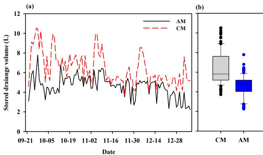
**Figure 5.** Changes in stored drainage volume in the drainage tank (a) and box-plot comparison between conventional (CM) and alternative (AM) nutrient-replenishment methods (b) during the experimental period.
