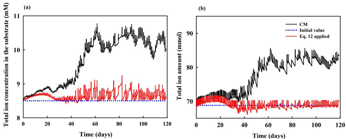
**Figure 2.** Changes in total ion concentration in the substrate (a) and total ions in the system (b) in the closed-loop soilless culture system using conventional (CM) and alternative (Equation (12) applied) nutrient-replenishment methods.
