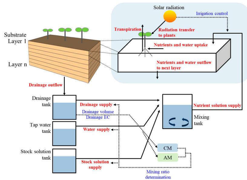
**Figure 1.** Schematic description of a closed-loop soilless culture system in a simulated condition. Solid lines indicate water and nutrient flow, and dotted lines indicate data flow for nutrient solution mixing and irrigation control. CM and AM mean conventional and alternative nutrient-replenishment methods, respectively.
