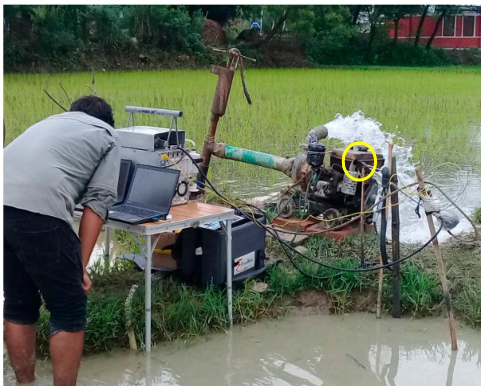
**Figure 3.** Real-time measurement of pump emissions in a paddy field, Saptari district, Nepal. Yellow circle indicates Ratnoze1 inlet near to the pump exhaust.
