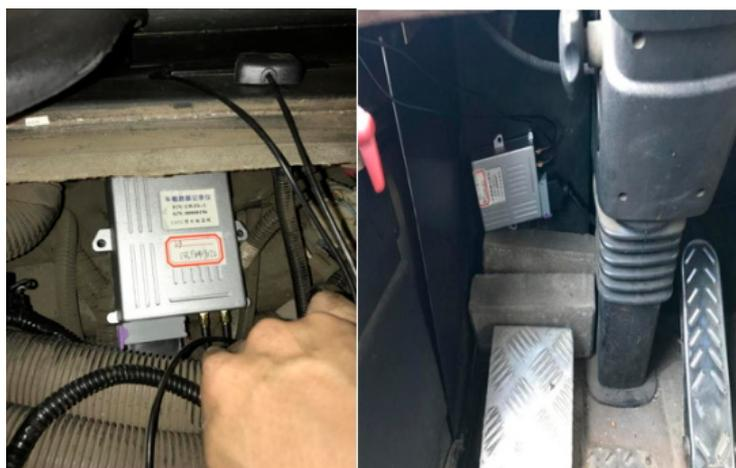
**Figure 1.** Vehicle engine data logger.
