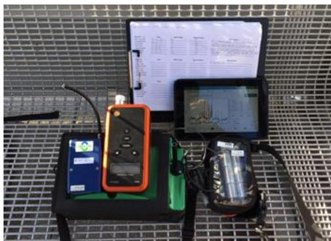
Figure 4. Devices set up for train/outdoor platform for “light measurements”.
