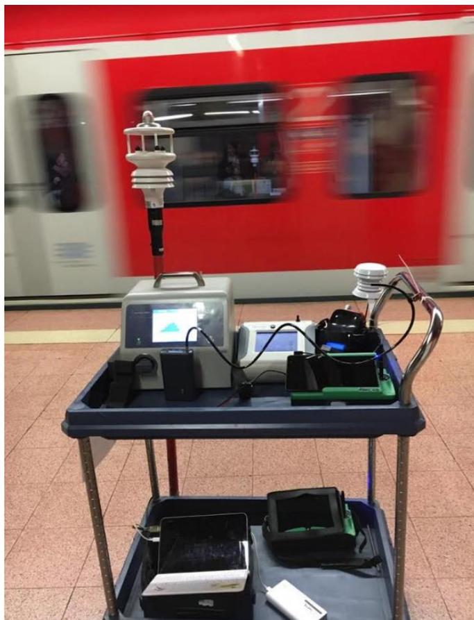
**Figure 3.** Devices set up for underground platform measurements.
