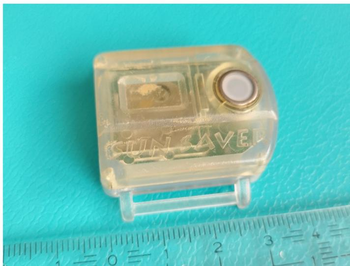
**Figure 1.** Electronic miniature UV-meter of the Sunsafer type [27].
