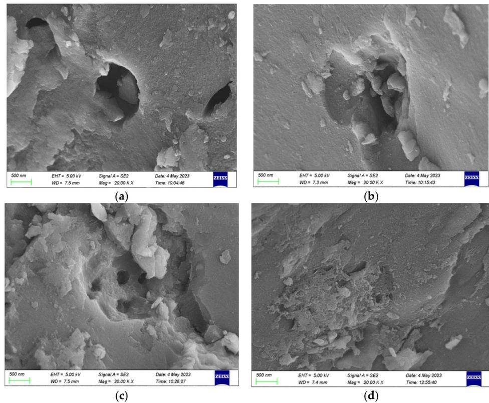
**Figure 1.** Schematic diagrams of SEM images of coal samples: (a) raw coal; (b) coal treated with 1 wt% [Bmin]Cl solution; (c) coal treated with 3 wt% [Bmin]Cl solution; (d) coal treated with 5 wt% [Bmin]Cl solution.
