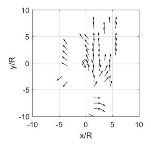
**Figure 8.** A composite of all of the data considered by Young [31] showing the mean values of the dominant wave direction in squares of size  $1R \times 1R$ . Areas with no vectors shown correspond to squares where there were insufficient measurements to form a reliable estimate of dominant wave direction. The tropical cyclone centre is shown by the open circle at co-ordinates (0, 0). The system is shown for the Northern Hemisphere (i.e., anti-clockwise circulation).
