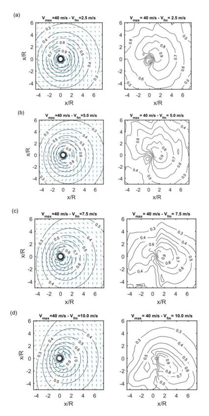
**Figure 5.** Tropical cyclone wind fields (left) and wave fields (right). The wind is calculated from the Holland vortex [1] and the waves from the results of Young [43]. The contours show normalized wind speed  $U_{10}/V_{\text{max}}$  (left) and normalized wave height  $H_s/H_s^{\text{max}}$  (right). Each of the panels (**a**–**d**) are for a different combination of  $V_{fm}$  and  $V_{\text{max}}$ , as marked.
