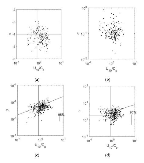
**Figure 7.** Spectral parameters for the one-dimensional form (12) as determined by Young [31]. (a) top left—spectral decay, *n*, with n = -4 shown, (b) top right—spectral width,  $\sigma$ , (c) bottom left—scale parameter,  $\beta$ , with relationship (13), (d) bottom right—peak enhancement,  $\gamma$ , with relationship (14).
