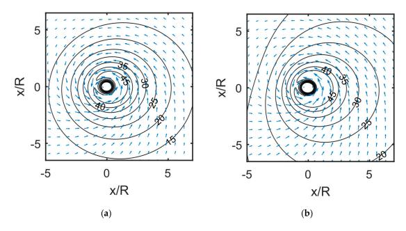
**Figure 1.** Tropical cyclone wind fields. (a) Left panel—calculated with a single Holland vortex (1) and parameters,  $p_0 = 950$  HPa,  $p_n = 1005$  HPa, R = 30 km, B = 1.75 and  $V_{fm} = 5$  ms<sup>-1</sup> (b) Right panel—calculated with a double Holland vortex and parameters,  $p_{0_1} = 955$  HPa,  $p_{0_2} = 1000$  HPa,  $R_1 = 30$  km,  $R_2 = 300$  km,  $B_1 = 1.75$  and  $B_2 = 2.2$ .
