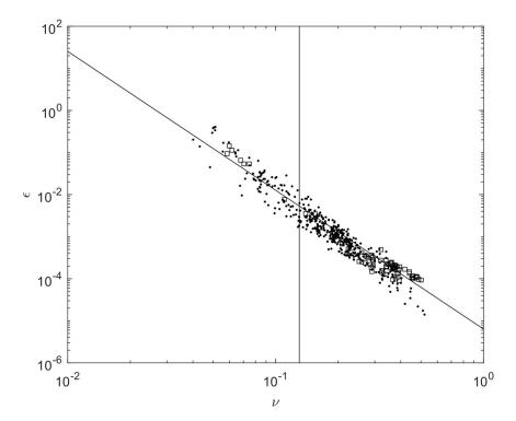
**Figure 3.** Values of the non-dimensional energy,  $\varepsilon$  as a function of non-dimensional peak frequency,  $\nu$ . The buoy data of Young [30,31] are shown by the solid dots and the aircraft based Hurricane Hunter data [48–51] by the open squares. The vertical line makes the commonly adopted division between swell (left of line) and wind-sea (right of line).
