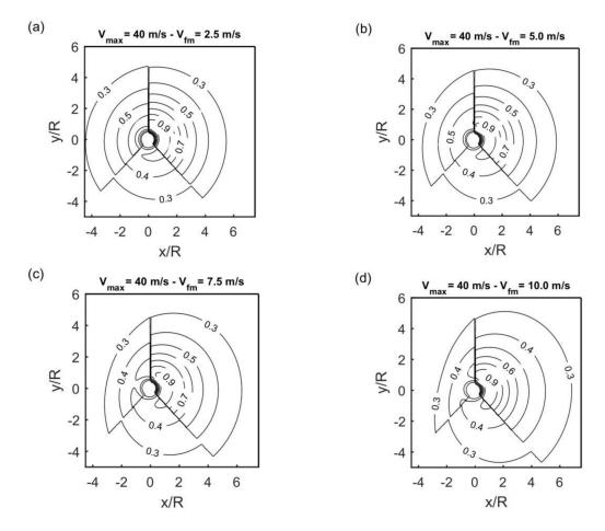
**Figure 6.** Tropical cyclone wave fields, calculated from the model of Hwang [48] and Hwang and Walsh [49]. Contours are of  $H_s/H_s^{max}$ . Each of the panels (**a**) to (**d**) is for a different combination of  $V_{fm}$  and  $V_{max}$ , as marked.
