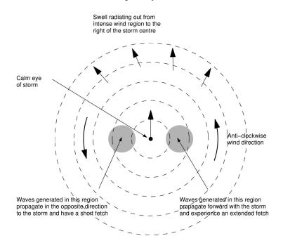
**Figure 2.** Schematic diagram showing the generation of waves within a translating northern hemisphere tropical cyclone. The tropical cyclone shown is translating "up the page", as shown by the arrow at the centre of the storm. The wave field is characterized by (i) swell ahead of the storm, radiating out from the intense wind region to the right of the storm centre, and (ii) significant asymmetry caused by the higher winds and extended translating fetch to the right of the storm centre.
