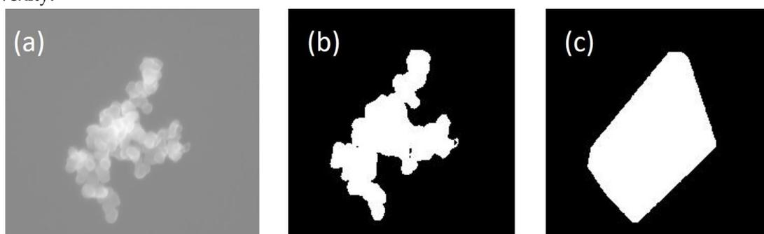
**Figure S2.** Calculation of convexity: (a) original Scanning Electron Microscopy (SEM) image, (b) 2D projected area of aggregate (c) convex polygon around aggregate.
