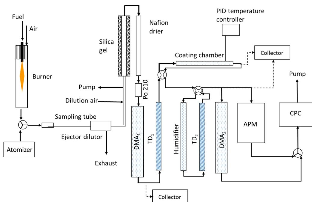
**Figure S1.** An integrated system for aerosol generation, processing, and analysis
