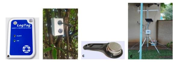
**Figure 2.** Meteorological instrument installations. Note: (a) Logtag recorder; (b) Logtag recorder installation in the box; (c) Ibutton data logger; and (d) meteorological micro-station HOBO.
