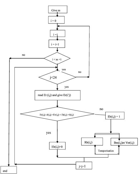
Figure 4. Algorithm of optimal leaks management.
