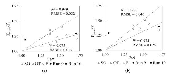
**Figure 4.** Effect of flow contraction on additional scour components using (a) Colorado State University (CSU) and (b) Melville-Sheppard (M/S) equations.
