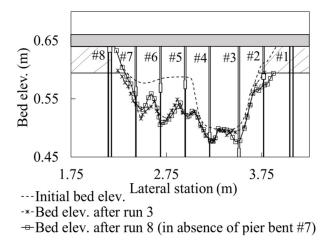
**Figure 6.** Comparison of cross-sections for runs 3 and 8.
