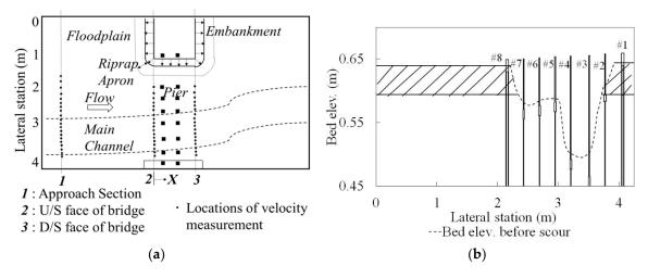
**Figure 2.** Geometry of compound channel for (a) plan view with velocity measurement locations; (b) cross section view at bridge.
