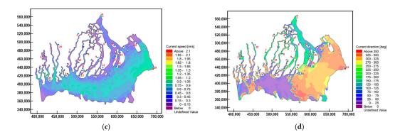
**Figure 8.** Spatial variation at spring tide on 22 August 2009 at 2:55 p.m. (a) surface elevation (EL + m); (b) total water depth (m); (c) current speed (m/s); and (d) current direction (degree).
