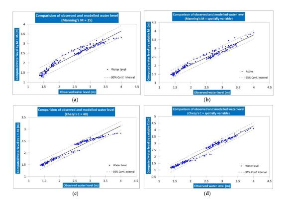
**Figure 5.** The goodness of fit for the rainy season, (a) water level by constant Manning m vs. observed water level and (b) variable Manning's m vs. observed, (c) constant Chezy c vs. observed and (d) variable Chezy c vs. observed water level at Chandpur station.
