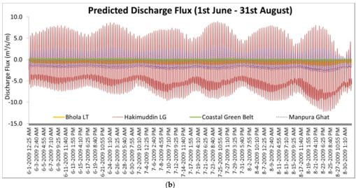
**Figure 7.** Discharge fluxes of the Meghna river estuary (a) Chandpur, Mehendiganj LG and Dashmina (b) Bhola LT, Hakimuddin LG, Coastal Green Belt and Manpura Ghat.
