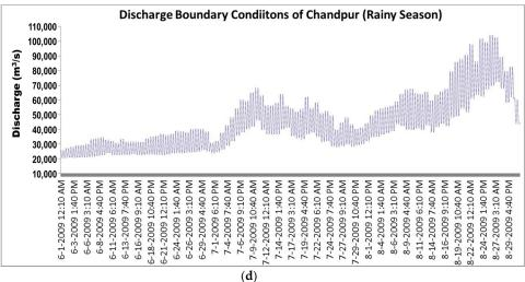
**Figure 3.** Boundary conditions (**a**) tide level in dry season; (**b**) tide level in rainy season at Chittagong station; (**c**) discharge in dry season; and (**d**) discharge in rainy season at Chandpur station.
