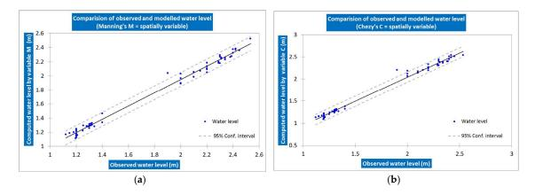
**Figure 4.** The goodness of fit for the dry season, (a) water level calculated by Manning's equation vs. observed water level and (b) water level calculated by the Chezy equation vs. observed water levels at Chandpur station.
