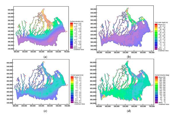
**Figure 9.** Spatial variation at neap tide on 23 August 2009 at 10:40 p.m. (**a**) surface elevation (EL + m); (**b**) total water depth (m); (**c**) current speed (m/s); and (**d**) current direction (degree).
