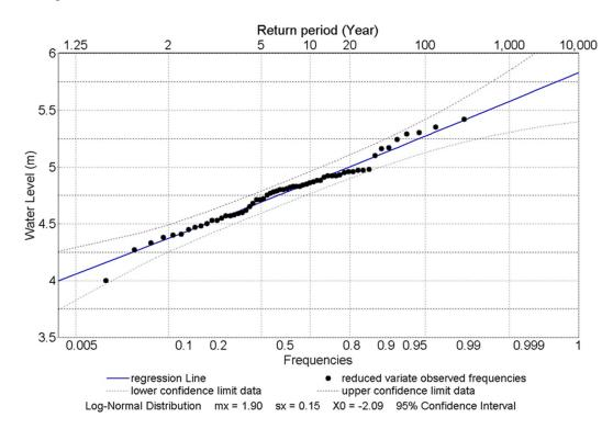
**Figure 13.** Water level returning period and frequencies for water level prediction at the downstream Chittagong station.
