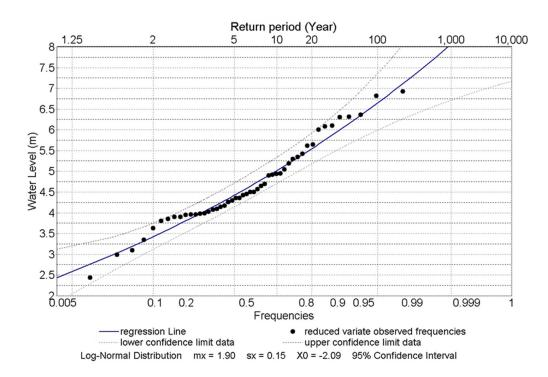
**Figure 12.** Water level returning period and frequencies for water level prediction at the upstream Chandpur station.
