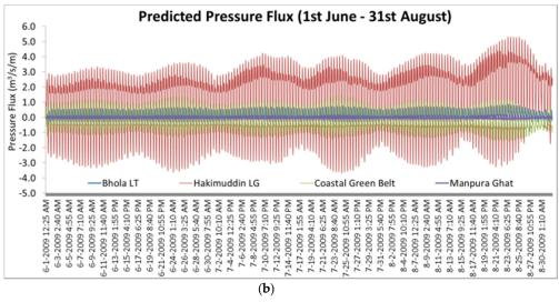
**Figure 6.** The variation of pressure flux for the un-gauged stations of Meghna river estuary (a) Mehendiganj LG and Dashmina (b) Bhola, Hakimuddin, Coastal Green Belt and Manpura Ghat.
