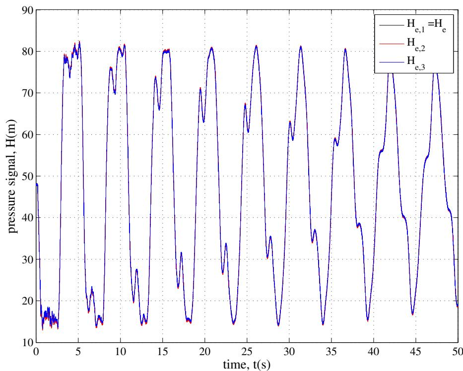
**Figure 4.** Trento TM: transient tests generated by pump shutdown. Note that the behavior of the pressure signals testifies the repeatability of tests.
