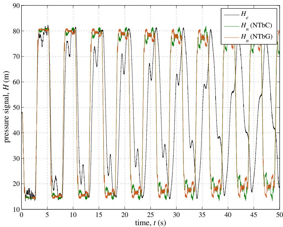
**Figure 7.** Trento TM: transient generated by pump shutdown at the well-field. Experimental pressure signal,  $H_e$ , at section M vs. model simulation,  $H_n$ , for the system with only branch C (NTbC), and only branch G (NTbG).
