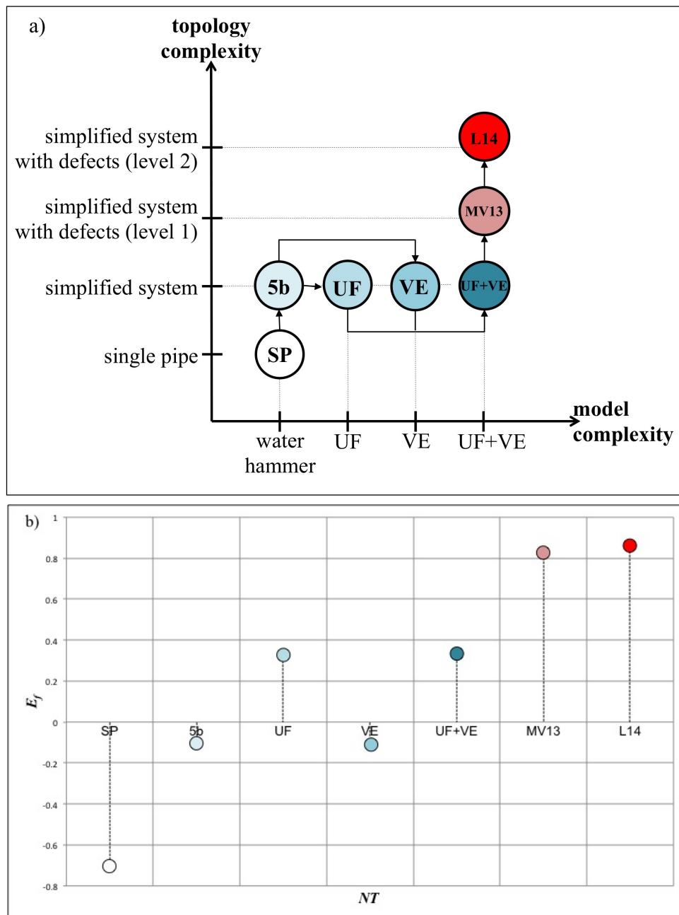
**Figure 14.** Procedure within the numerical model implementation for evaluating the relevance of the topology simulation (a) and model complexity in the transient response of the TM (b).
