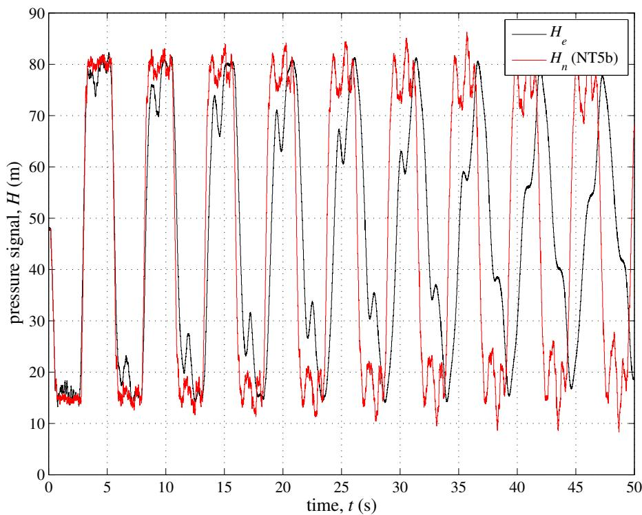
**Figure 8.** Trento TM: transient generated by pump shutdown at the well-field. Experimental pressure signal,  $H_e$ , at section M vs. model simulation,  $H_n$ , for the system with 5 branches (B, C, E, G and I) selected by means of the value of  $E_f$  (NT5b).
