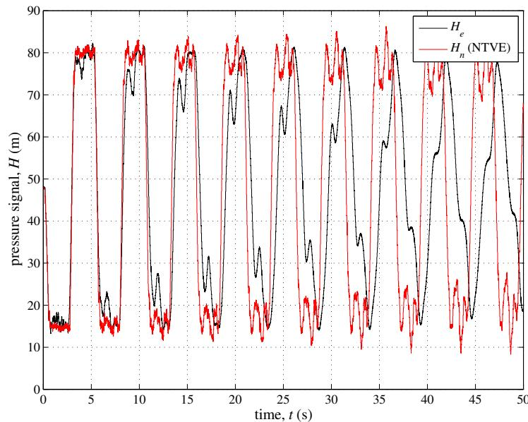
**Figure 10.** Trento TM: transient generated by pump shutdown at the well-field. Experimental pressure signal,  $H_e$ , at section M vs. model simulation,  $H_n$ , for the system with the 5 branches (B, C, E, G and I) and the viscoelasticity (for branch E, with  $L_{b,E} = L_{b,E'}$ ) included in the model (NTVE).
