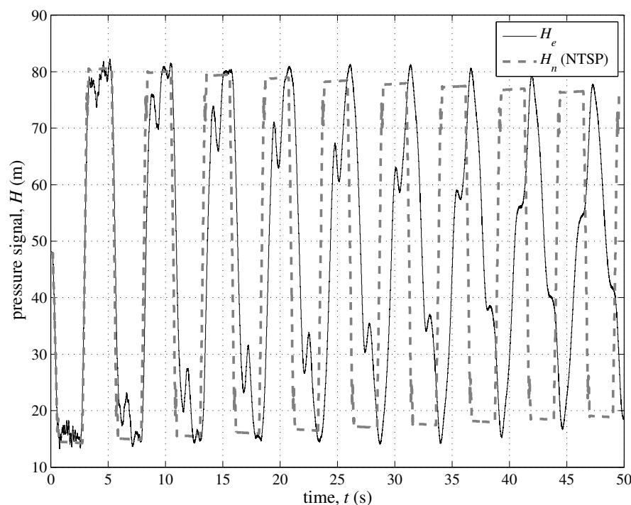
**Figure 5.** Trento TM: transient generated by pump shutdown at the well-field. Experimental pressure signal,  $H_e$ , at section M vs. model simulation,  $H_n$ , for the single pipe scheme (NTSP).
