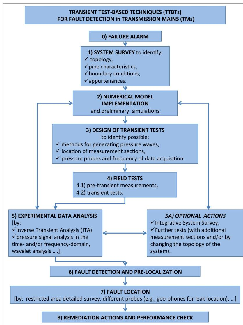
**Figure 1.** Transient test-based techniques (TTBTs) for fault detection in Transmission Mains (TMs): main phases of the procedure with highlighted the interactions between them.
