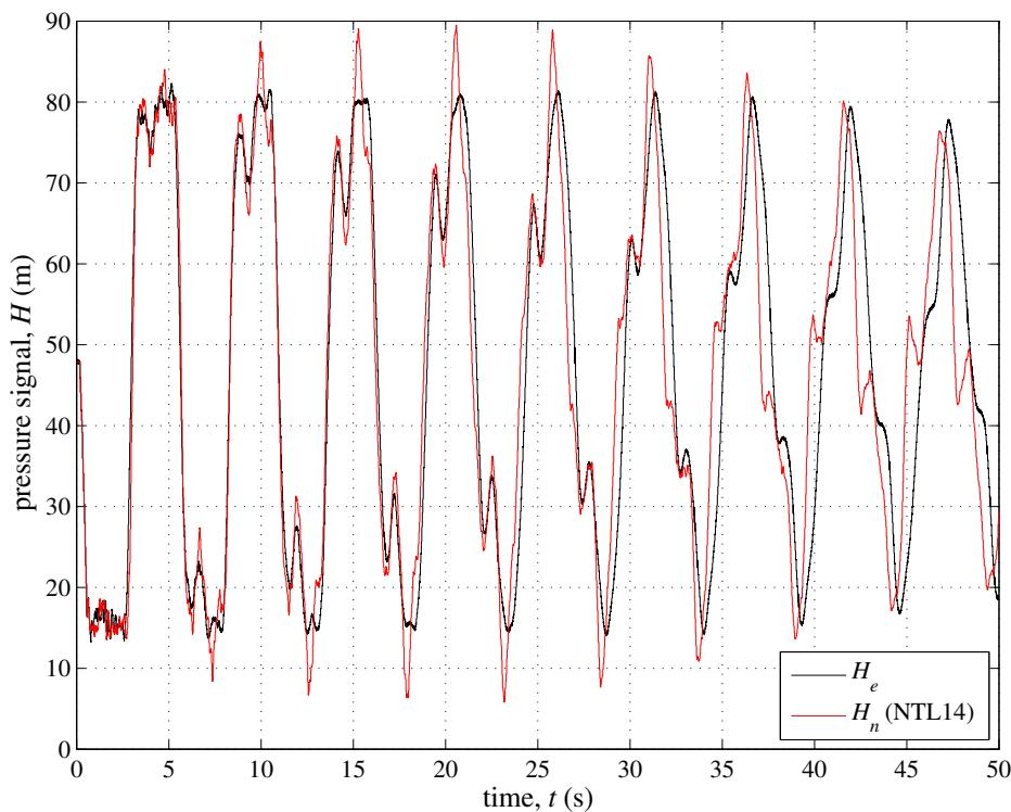
**Figure 13.** Trento TM: transient generated by pump shutdown at the well-field. Experimental pressure signal,  $H_e$ , at section M vs. model simulation,  $H_n$ , for the system with the 5 branches B, C, E, G, and I, the unsteady friction and the viscoelasticity (for branch E, with  $L_{b,E} = L_{b,E'} + L_{b,E''}$ ) included in the model, and a small leak,  $Q_L$ , at node 14 (NTL14).
