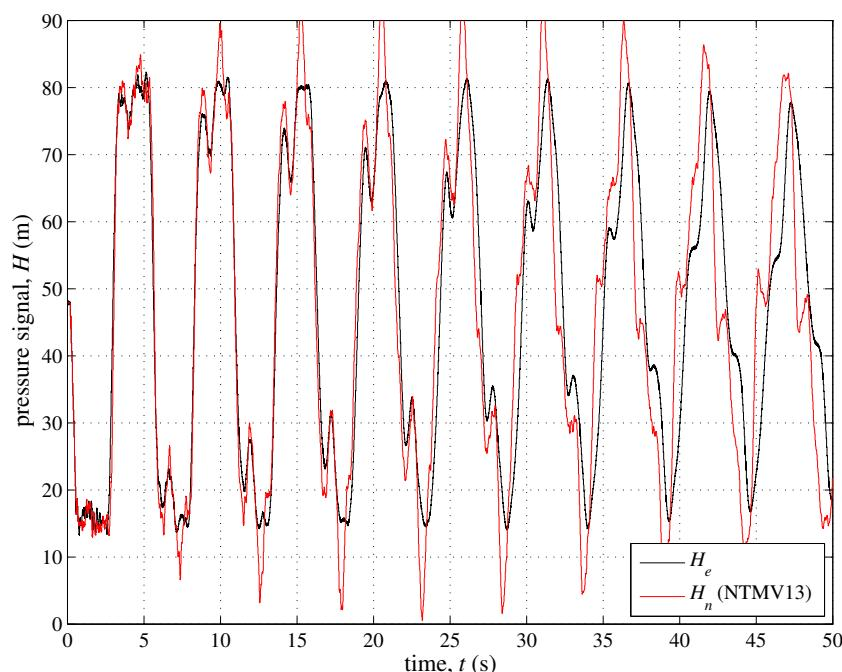
**Figure 12.** Trento TM: transient generated by pump shutdown at the well-field. Experimental pressure signal,  $H_e$ , at section M vs. model simulation,  $H_n$ , for the system with the 5 branches B, C, E, G, and I, the unsteady friction and the viscoelasticity (for branch E, with  $L_{b,E} = L_{b,E'} + L_{b,E''}$ ) included in the model, and a malfunctioning valve at node 13 (NTMV13).
