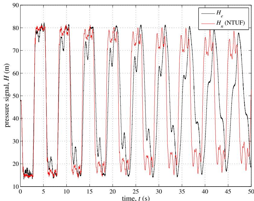
**Figure 9.** Trento TM: transient generated by pump shutdown at the well-field. Experimental pressure signal,  $H_e$ , at section M vs. model simulation,  $H_n$ , for the system with the 5 branches (B, C, E, G and I) and the unsteady friction included in the model (NTUF).
