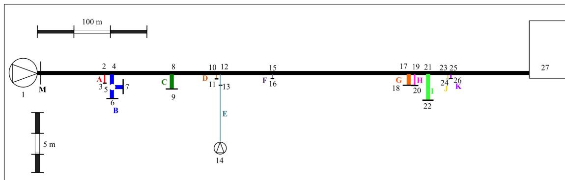
**Figure 3.** Trento TM layout (note that letters indicate the branches, whereas numbers indicate the nodes of the system; in particular: 1—well-field; M—measurement section; 27—downstream end reservoir; a different length scale has been used for the main pipe and minor branches).
