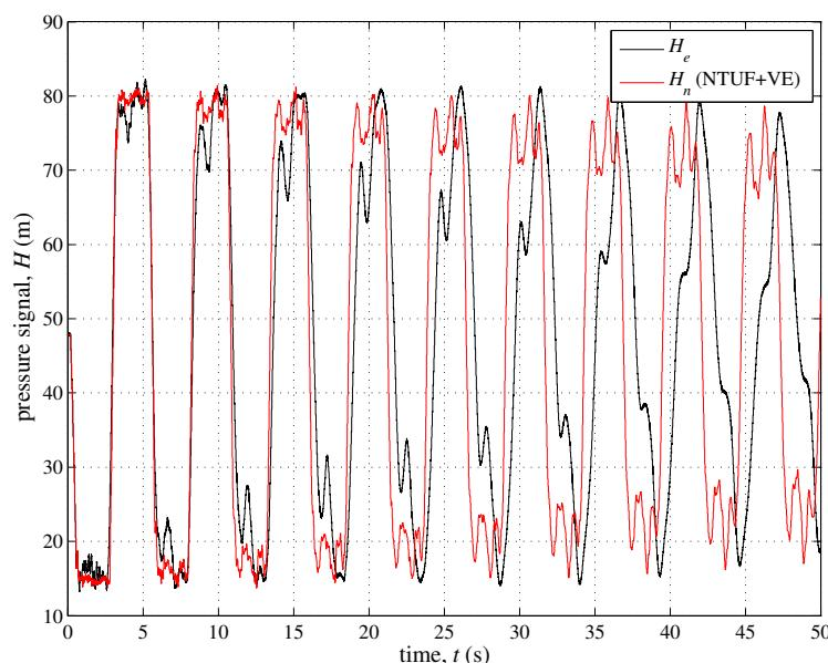
**Figure 11.** Trento TM: transient generated by pump shutdown at the well-field. Experimental pressure signal,  $H_e$ , at section M vs. model simulation,  $H_n$ , for the system with the 5 branches (B, C, E, G and I) and both the unsteady friction and the viscoelasticity (for branch E, with  $L_{b,E} = L_{b,E'}$ ) included in the model (NTUF + VE).
