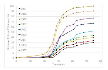
**Figure 7.** Sediment release efficiency from 2013 to 2037 as computed from measurements in the physical model.
