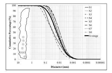
Figure 4. Grain size distribution from samples collected in the lower Wushe Reservoir.
