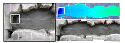
Figure 8. Ultimate depositional pattern of the Wushe Reservoir.
