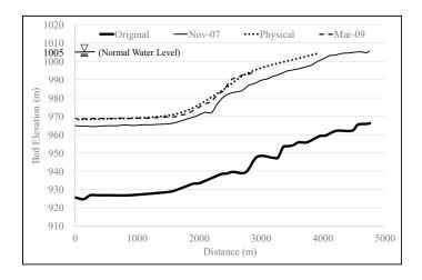
Figure 5. Longitudinal bed elevation of the physical model and field-measured data.
