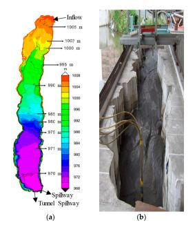
Figure 3. (a) Bed elevation of the Wushe Reservoir; (b) physical model.
