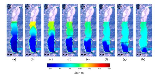
**Figure 6.** Deposition delta movement patterns from 2013 to 2034. (a) 2013; (b) 2016; (c) 2019; (d) 2022; (e) 2025; (f) 2028; (g) 2031; (h) 2034.
