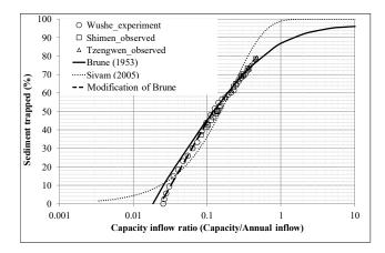
Figure 10. Relationship of the capacity inflow ratio and the trap efficiency.
