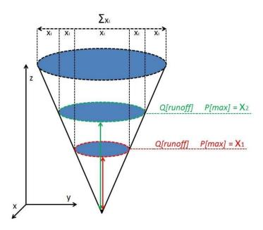
Figure 2. A representation of the relation between flooded area and amount of precipitation.
