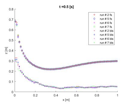
**Figure 4.** Comparison of free surface (fs) and mixture–water interface (bls) at the reference time t = 0.5 s. Limiting viscosity decreases from Run 2 to Run 6 according to Table 2.
