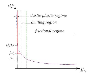
**Figure 1.** Apparent viscosity versus second invariant of the rate of deformation tensor: the blue dashed line refers to typical pseudoplastic behavior, while the red line refers to the non-Newtonian rheological behavior of the reference mixture model, as modified by the limiting viscosity.
