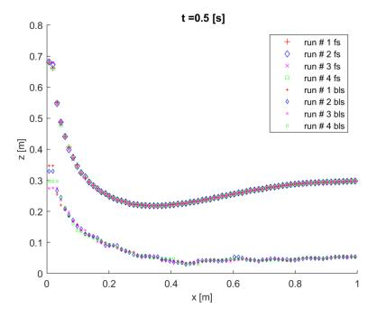
**Figure 3.** Comparison of free surface (fs) and mixture–water interface (bls) at the reference time t = 0.5 s. Threshold viscosity increases from Run 1 to Run 4 according to Table 1.
