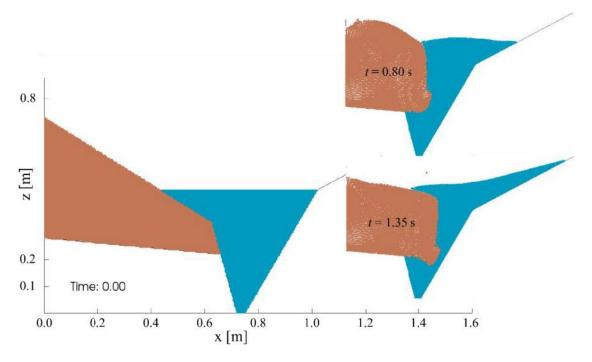
**Figure 6.** (Left) Sketch of the landslide toe and stored water from the Padua experiment; and (Right) frames at some significant time instants (ref. Run V1).
