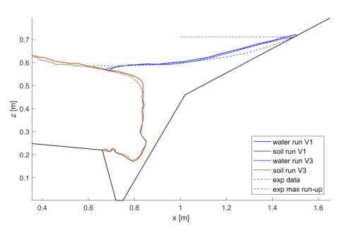
Figure 8. Comparison of maximum simulated run-up at t = 1.35 s for changes in the limiting viscosity.
