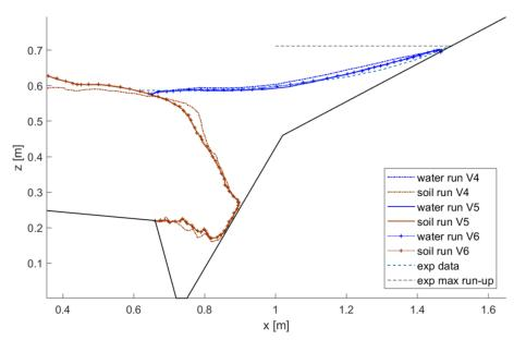
Figure 11. Comparison of maximum simulated run-up at t = 1.35 s for changes in spatial resolution dx.
