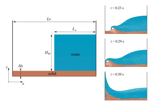
**Figure 2.** Computational domain of the 2D erosive dam break (initial time). Right-hand panels show the frames at some representative time instants (Ref. Run 2).
