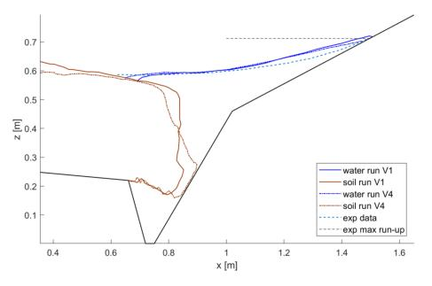
Figure 9. Comparison of maximum simulated run-up at t = 1.35 s for changes in saturation.
