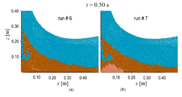
**Figure 5.** Magnification of the maximum sediment run-up: (**a**) Run 6; and (**b**) Run 7. Light brown solid particles in the right-hand panel are in the elastic–plastic regime (fixed).
