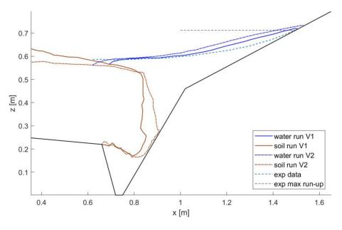
Figure 7. Comparison of maximum simulated run-up at t = 1.35 s for change in the angle of internal friction.
