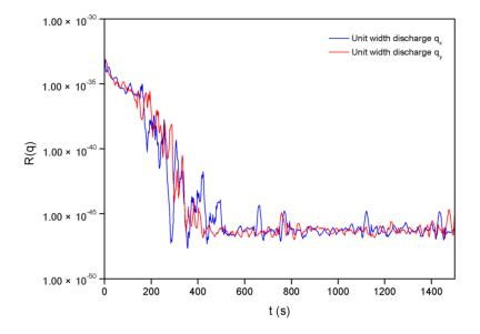
Figure 7. Global relative errors of unit width discharges in *x* and *y* directions.
