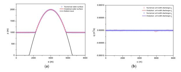
**Figure 6.** Comparisons between numerical and analytical results at t = 1500 s: (**a**) water surface; (**b**) unit width discharges in *x* and *y* directions.
