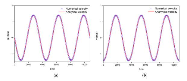
**Figure 12.** Comparison between simulated and analytical velocities for the mesh of  $\Delta L = 55.18$  m at the point (-5000, -100): (**a**) *u* velocity; (**b**) *v* velocity.
