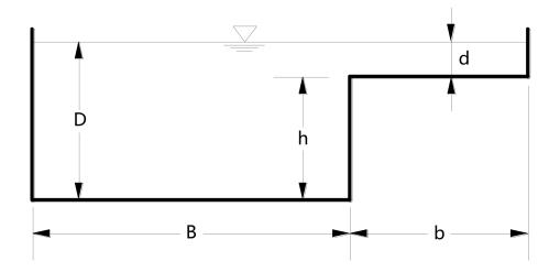
Figure 18. Sketch of a cross-section in a simplified compound channel.
