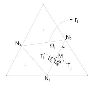
Figure 2. Notations of a typical triangular cell and its three neighbors.
