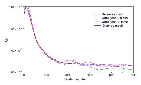
Figure 16. Global relative errors of water depth on different types of mesh.
