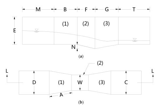
Figure 20. Sketch of the Parshall flume: (a) section view of L-L; (b) plan view.
