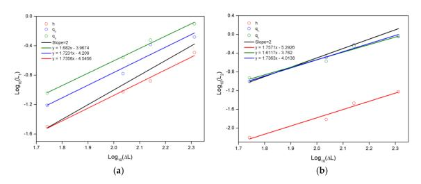
**Figure 14.** Errors of the numerical scheme in  $L_1$  and  $L_2$  norms at t = 3T for h,  $q_x$  and  $q_y$ : (a)  $L_1$  errors; (b)  $L_2$  errors.
