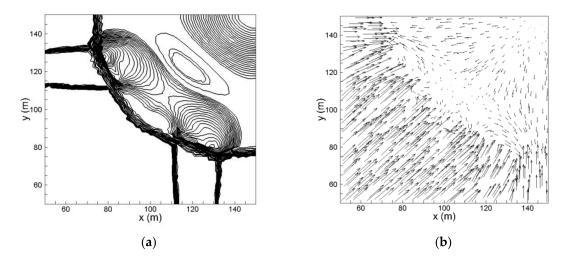
**Figure 24.** Numerical results of the 2D Riemann problem at t = 4 s: (a) contours of water surface elevation; (b) vector field of flow velocities.
