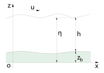
Figure 1. Sketch of shallow water flow over uneven topography.
