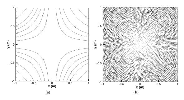
**Figure 9.** Numerical results of the potential flow test: (**a**) contours of water depth; (**b**) vector field of flow velocities.
