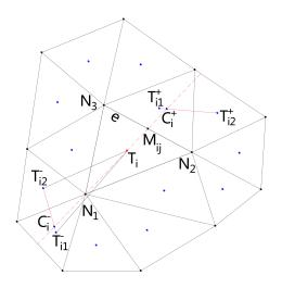
Figure 4. Sketch of Touze's scheme on triangular grids.
