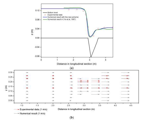
**Figure 21.** Comparison of experimental and simulated results along the flume: (**a**) water surface; (**b**) *x*-directional velocity.
