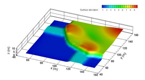
**Figure 23.** Simulated water surface of the 2D Riemann problem in 3D view at t = 4 s.
