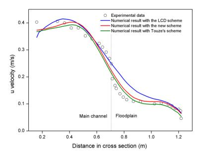
Figure 19. Comparison of experimental and simulated longitudinal velocities.
