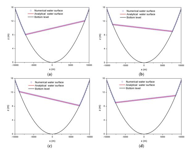
**Figure 11.** Comparison between simulated and analytical water surface for the mesh of  $\Delta L = 55.18$  m. (a) t = T; (b) t = T + T/3; (c) t = T + T/2; (d) t = 2T + T/6.
