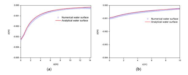
**Figure 17.** Comparisons between simulated and analytical water surface on the distorted mesh along: (a) the diagonal section; (b) the horizontal-symmetry section.
