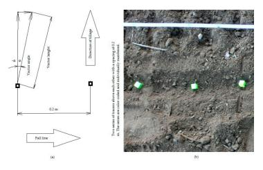
Figure 2. Design of tracers (location) before pass: (a) Description of measures; (b) One series of tracers.
