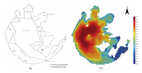
**Figure 1.** (a) Eight subzones, boundary discharge locations, cross-sections and positions of 5 monitoring stations, namely, 1. Wangting Station; 2. Dapukou Station; 3. Jiapu Station; 4. Xiaomeikou Station; 5. Xishan Station. (b) Grid and depth used in numerical model, depth unit: m.
