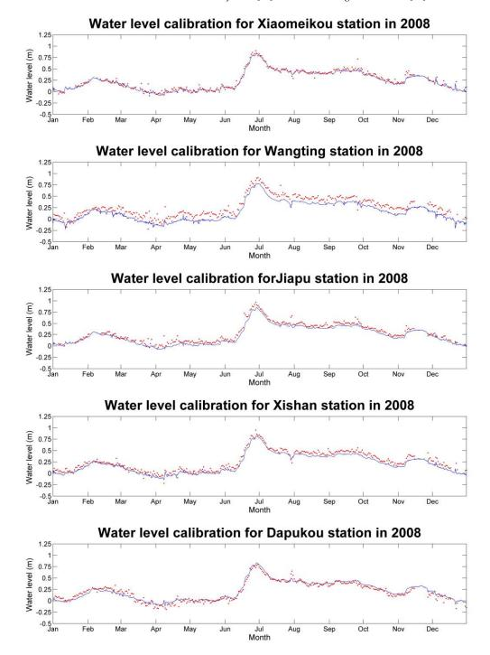
**Figure 3.** In situ measured and modeled water level for five monitoring stations in 2008, water levels are based on Wusong Datum. Measured levels are shown with points, and model results are shown with solid lines.
