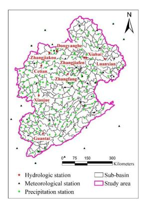
**Figure 2.** The distribution of the river net, sub-basins, and the locations of meteorological, precipitations and hydrologic stations which were used in the model simulations in HRB.
