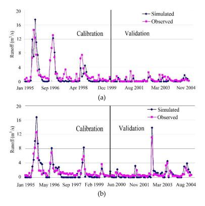
**Figure 4.** The comparison of the observed and simulated runoff at the Zhangjiakou station (**a**) and the Dongyanghe station (**b**) (1995–2004).
