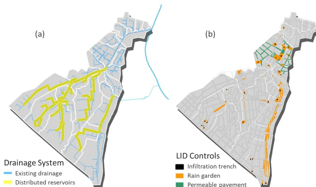
**Figure 2.** Proposed intervention measures: (a) distributed reservoirs under city roads; (b) low-impact development (LID) controls.
