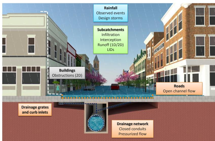
**Figure 3.** Schematic modeling representation for PCSWMM.
