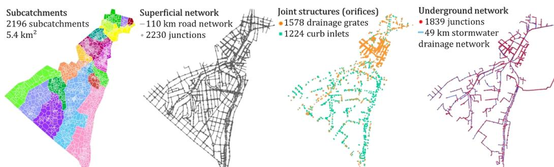
**Figure 4.** Modeling network for PCSWMM model and current drainage system.
