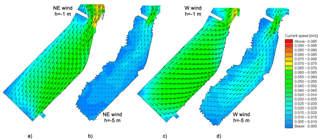
**Figure 12.** Hourly averaged current fields in the characteristic situations during an occurrence of barocline compensation currents in the area of the marina entrance, induced by (a,b) NE wind episode on 7 March 2017, 23:00 h, at a depth (a)  $h = -1$  m and (b)  $h = -5$  m; (c,d) W wind episode on 10 August, 17:00 h at a depth (c)  $h = -1$  m and (b)  $h = -5$  m.
