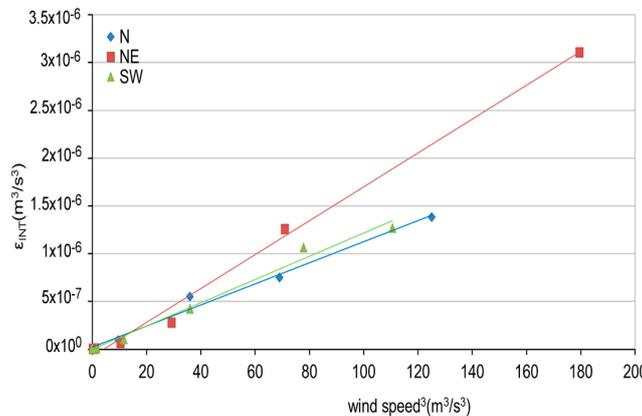
**Figure 14.** The integrated dissipation of turbulent kinetic energy through the vertical profile in the point of the marina centroid versus the cube of the wind speed for the N, NE and SW wind direction.
