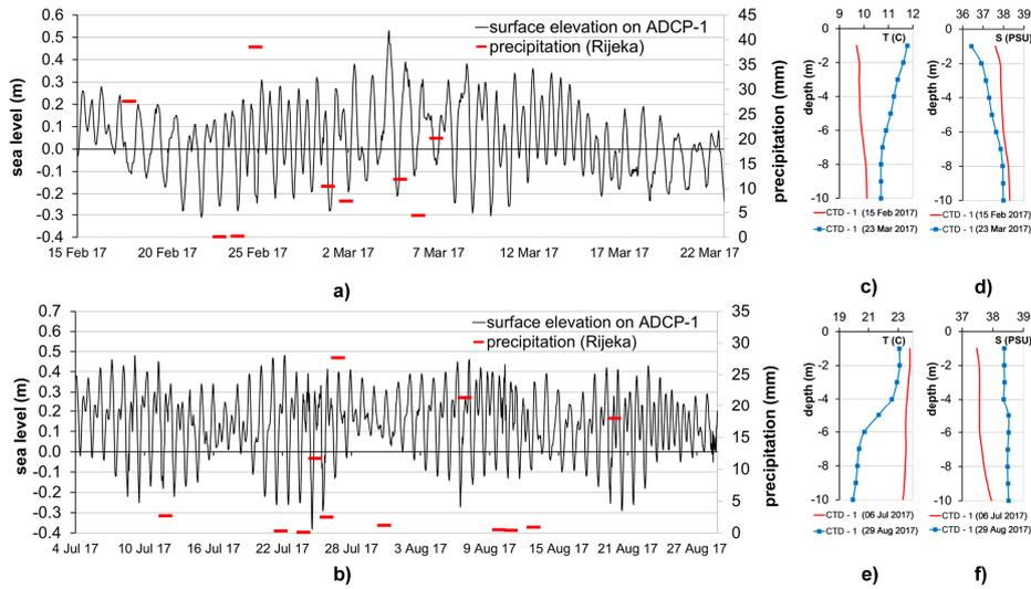
**Figure 4.** Time series of surface elevations recorded at the ADCP station 1 and daily precipitation at the meteorological station Rijeka ( $\phi = 45020'$ ,  $\lambda = 14027'$ ) for the (a) winter and (b) summer measurement periods; the sea temperature (T) and salinity (S) throughout the vertical sea column at site 1 for (c,d) the winter and (e,f) summer measurement periods.
