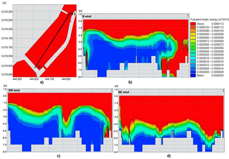
**Figure 13.** Turbulent kinetic energy field for the wind of 4.5 m/s speed trough vertical cross-section B1–B2: (a) the cross-section B1–B2 position; (b) TKE on 10th of March, 19:00 h for N wind; (c) TKE on 4th of March 22:00 h for SW wind; (d) TKE on 14th of July 10:00 h for NE wind.
