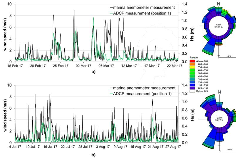
**Figure 5.** Time series of wind velocities and significant wave heights (measured at position 1, hourly averaged) with the corresponding wind rose for the (a) winter and (b) summer measurement periods.
