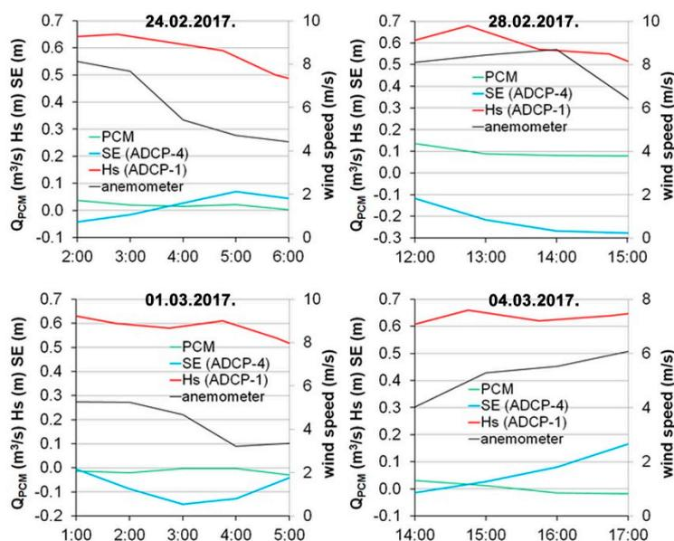
**Figure 21.** Hourly averaged field measured values of significant wave height ( $H_s$ ), surface elevation (SE), flushing culvert discharge measured with the PCM and wind velocity, during situations where the wave parameters were approximately equivalent.
