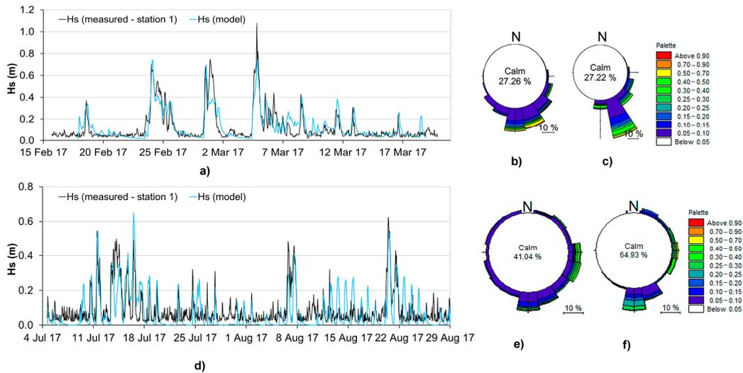
**Figure 19.** Comparison of measured and modelled time series of significant wave heights  $H_S$  at measurement station 1 for the (a) winter and (d) summer measurement periods with corresponding wave roses from (b,e) measured and (c,f) modelled data.
