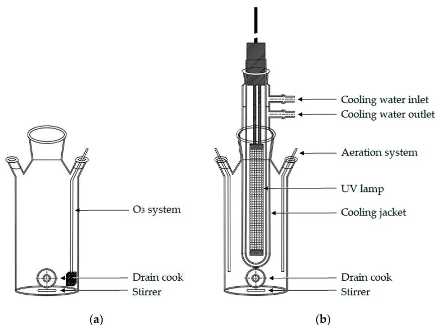
**Figure 1.** Reactor for the (a) H<sub>2</sub>O<sub>2</sub>, O<sub>3</sub>, and (b) UV, UV/TiO<sub>2</sub> [21] processes.
