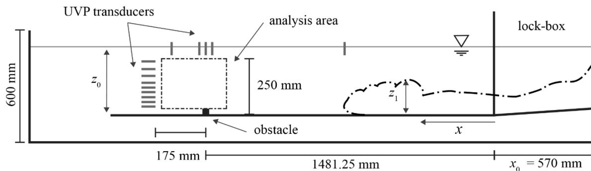
**Figure 4.** Elevation view of the unconfined basin, showing the UVP transducer configuration (labelled transducer #1–14, clockwise from bottom) and area of analysis, including the position of the square obstacle.
