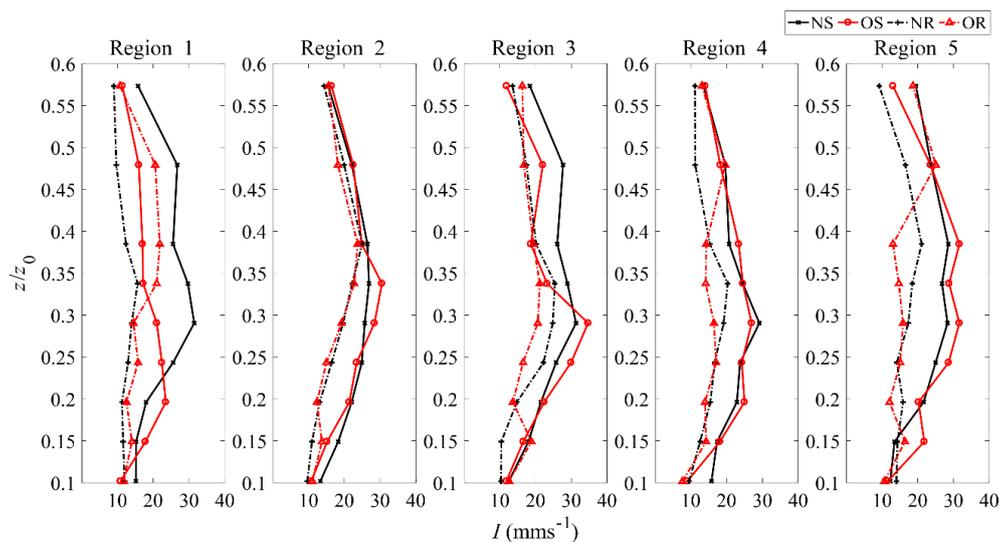
**Figure 12.** Non-dimensionalised vertical profiles of the horizontal turbulence intensity ( $I$ ) of all obstacle configurations for each allocated region of interest.
