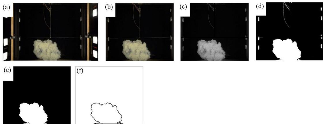
**Figure 6.** Step-by-step plan view of photometric image processing: (a) raw image; (b) cropped image adjusted for lens distortion; (c) greyscale conversion; (d) binary conversion; (e) removal of noise induced by the halogen lamps and UVP rack; and (f) delineated current boundary.
