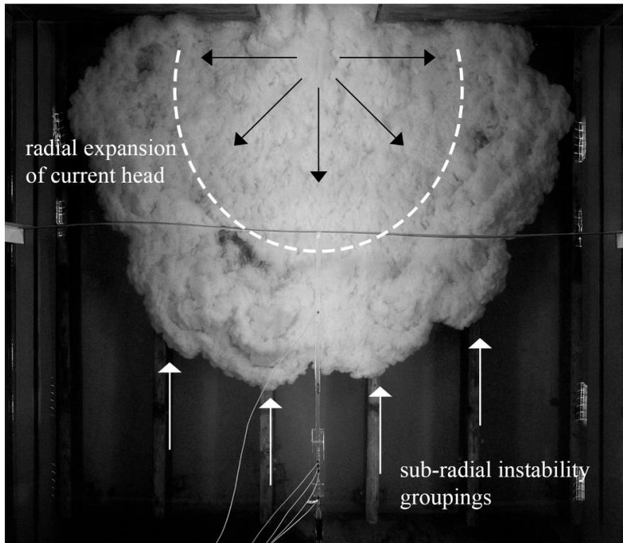
**Figure 10.** Example plan images of the current in test NS. The unconfined nature of the basin causes the current to expand in a radial movement upon release. The current head appears well-defined, where it is seen to detach from the current body in various locations. Current front intensities are also seen to form sub-radial groups for a smooth bed.
