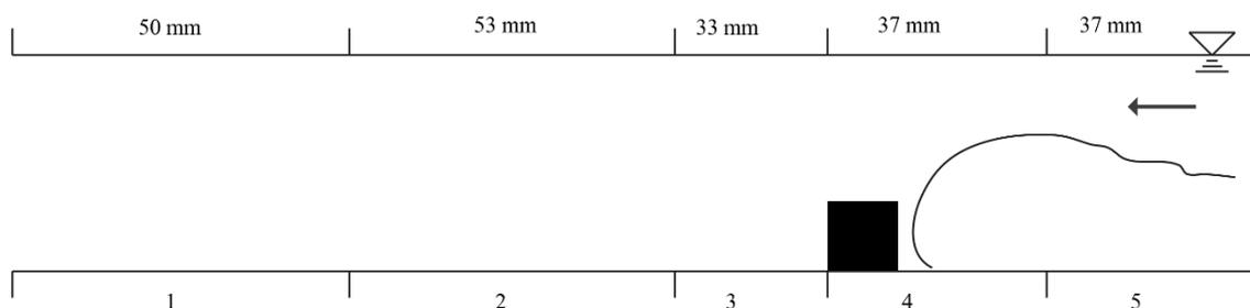
**Figure 7.** Elevation view of the five regions within the analysis area used for the velocity and turbulence intensity profile analysis. The regions were based on [12], with region widths optimized according to visible trends in non-averaged turbulence intensity plots.
