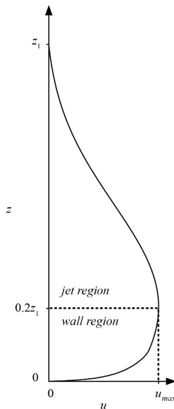
**Figure 1.** Typical velocity profile of an unobstructed gravity current, where velocity within the lower wall region represents a logarithmic shape and velocity in the upper jet region represents a Gaussian shape.
