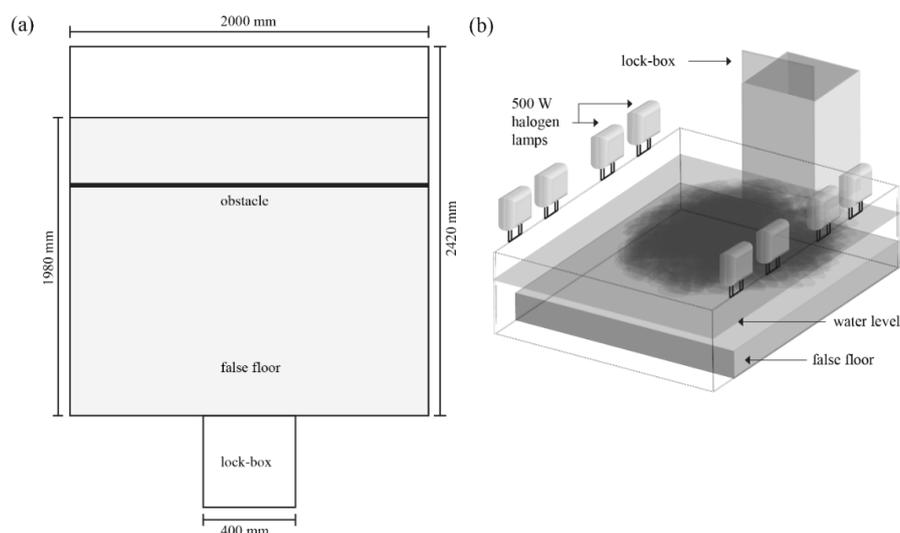
**Figure 2.** (a) Schematic plan view of the laboratory basin, including the location of the square cylindrical obstacle and false floor; (b) Illumination and lock-box configuration within the basin.
