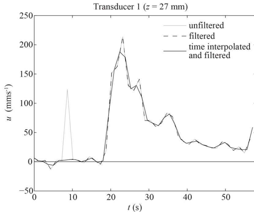
**Figure 5.** Time-series plot of velocities for channel 58 of transducer #1, comparing the unfiltered, raw data to filtered (with a standard deviation filter) and a combination of filtered/time interpolated data.
