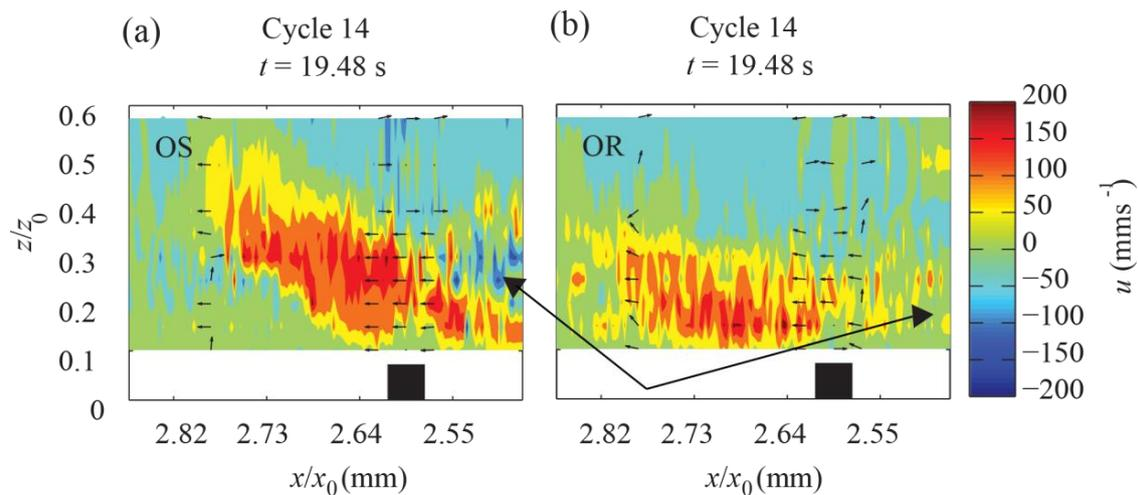
**Figure 9.** Non-dimensionalised spatial velocity contour plots (obtained from UVP) comparing the arrival of the current head in the analysis area for both smooth (a) and rough (b) bed conditions. The current head is characterized by a forward velocity below a faint ambient reverse flow. Regions of reverse flow are present directly behind the head for test OS but not OR.
