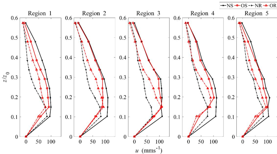
**Figure 8.** Non-dimensionalised vertical profiles of the horizontal velocity ( $u$ ) of all obstacle configurations for each allocated region of interest, where  $u$  has been averaged, per region, for each transducer.
