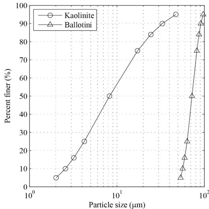
**Figure 3.** Grainsize distribution of the kaolinite clay and Ballotini spherical glass beads, the sedimentary compounds used to create the turbidity current slurry.
