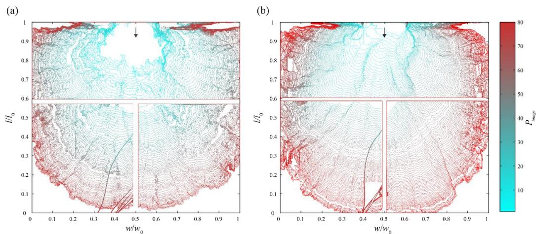
**Figure 11.** Spatially non-dimensionalised plan velocity contour plots from photometric analysis showing the progression of the current over the smooth substrate (a) and rough substrate (b).  $l_0$  and  $w_0$  represent the length and width of the image analysis area, respectively.  $P_{image}$  represents the consecutive image number recorded after opening of the lock-box. The black arrows signify flow direction.
