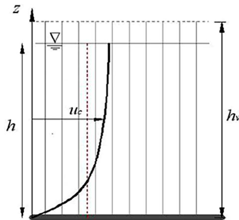
Figure 2. Flow over unsubmerged rigid vegetation.
