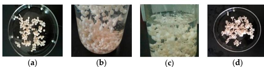
**Figure 3.** Microbial beads at different PVA concentrations. (a) 8% PVA; (b) 9% PVA; (c) 10% PVA; (d) 11%PVA.
