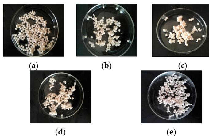
**Figure 4.** Microbial beads at different concentrations of sodium alginate (SA). (a) 0.25% SA; (b) 0.5% SA; (c) 1% SA; (d) 2% SA; (e) 3% SA.
