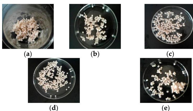
**Figure 5.** Microbial beads at different microbial biomass. (a) 5% biomass; (b) 7.5% biomass; (c) 10% biomass; (d) 12.5% biomass; (e) 15% biomass.
