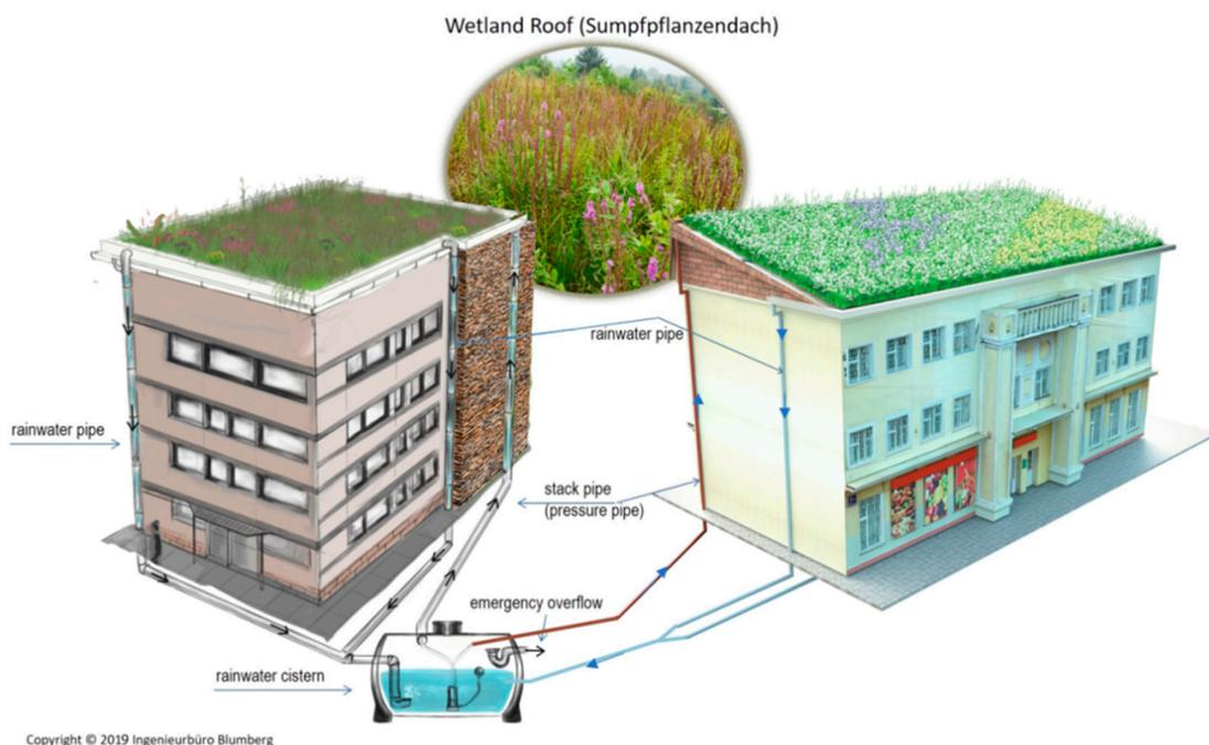
**Figure 3.** Buildings with wetland roofs for rainwater retention, evapotranspiration or for greywater treatment (graphic: Michael Blumberg).
