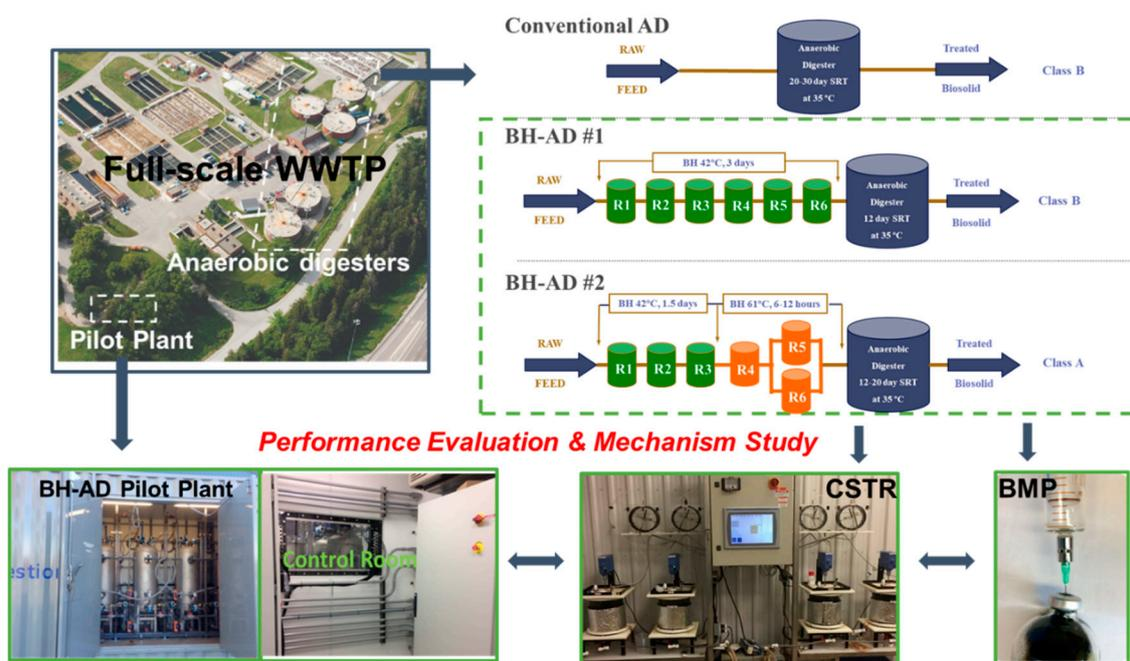
**Figure 1.** Biological hydrolysis–anaerobic digestion (BH-AD) process flow design and performance evaluation.
