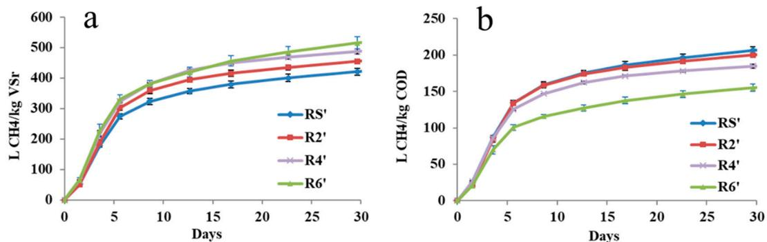
**Figure 3.** Methane yields of BH42-pretreated sludge by biochemical methane potential (BMP) tests: (a) methane yields ( $M1$ ) based on VS removal in the substrate ( $L\ CH_4/kg\ VSr$ ); (b) methane yields ( $M2$ ) based on initial total COD of the substrate ( $L\ CH_4/kg\ TCOD$ ). (the methane yields have been normalized at standard temperature and pressure (STP); RS': raw sludge; R2': BH at 42 °C for 24 h; R4': BH at 42 °C for 48 h; R6': BH at 42 °C for 72 h as listed in Table 1).
