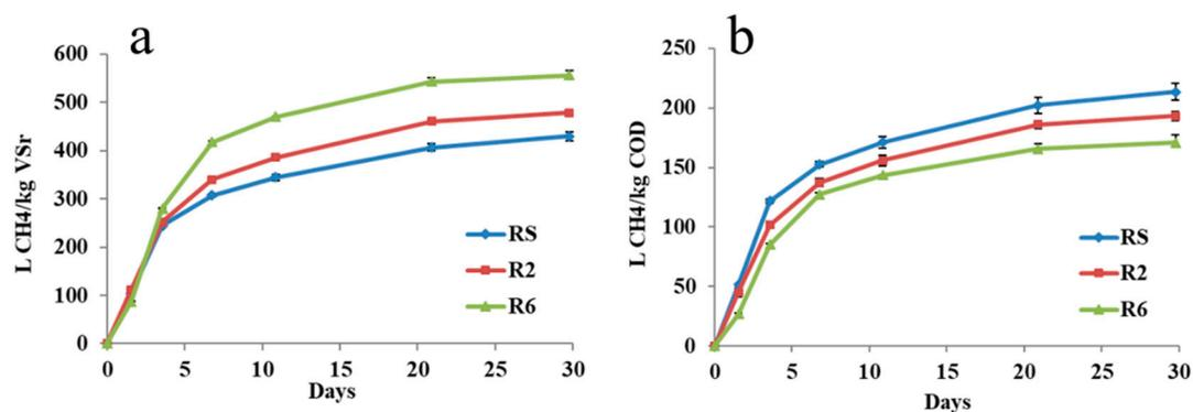
**Figure 4.** Methane yields of BH61 pretreated sludge by biochemical methane potential (BMP) tests: (a) methane yields ( $M1$ ) based on VS removal in the substrate ( $L\ CH_4/kg\ VSr$ ); (b) methane yields ( $M2$ ) based on initial total COD (kg COD) of the substrate ( $L\ CH_4/kg\ TCOD$ ). (the methane yields have been normalized at STP; RS: raw sludge; R2: BH at 42 °C for 36 h; R6: BH at 42 °C for 36 h and then 61 °C for 6 h as listed in Table 1).
