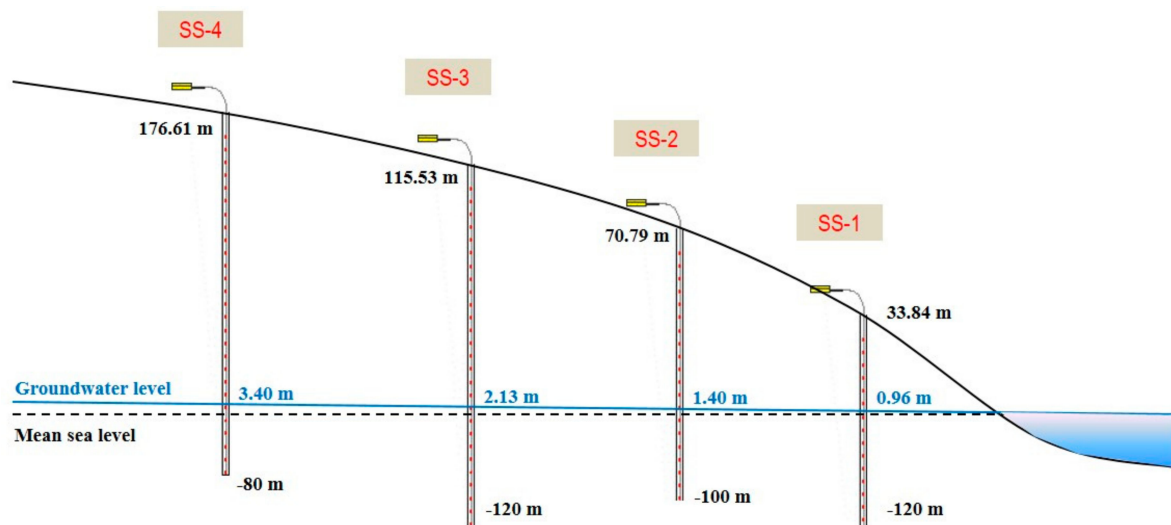
Figure 5. Schematic diagram of temperature monitoring using thermal line sensor system.
