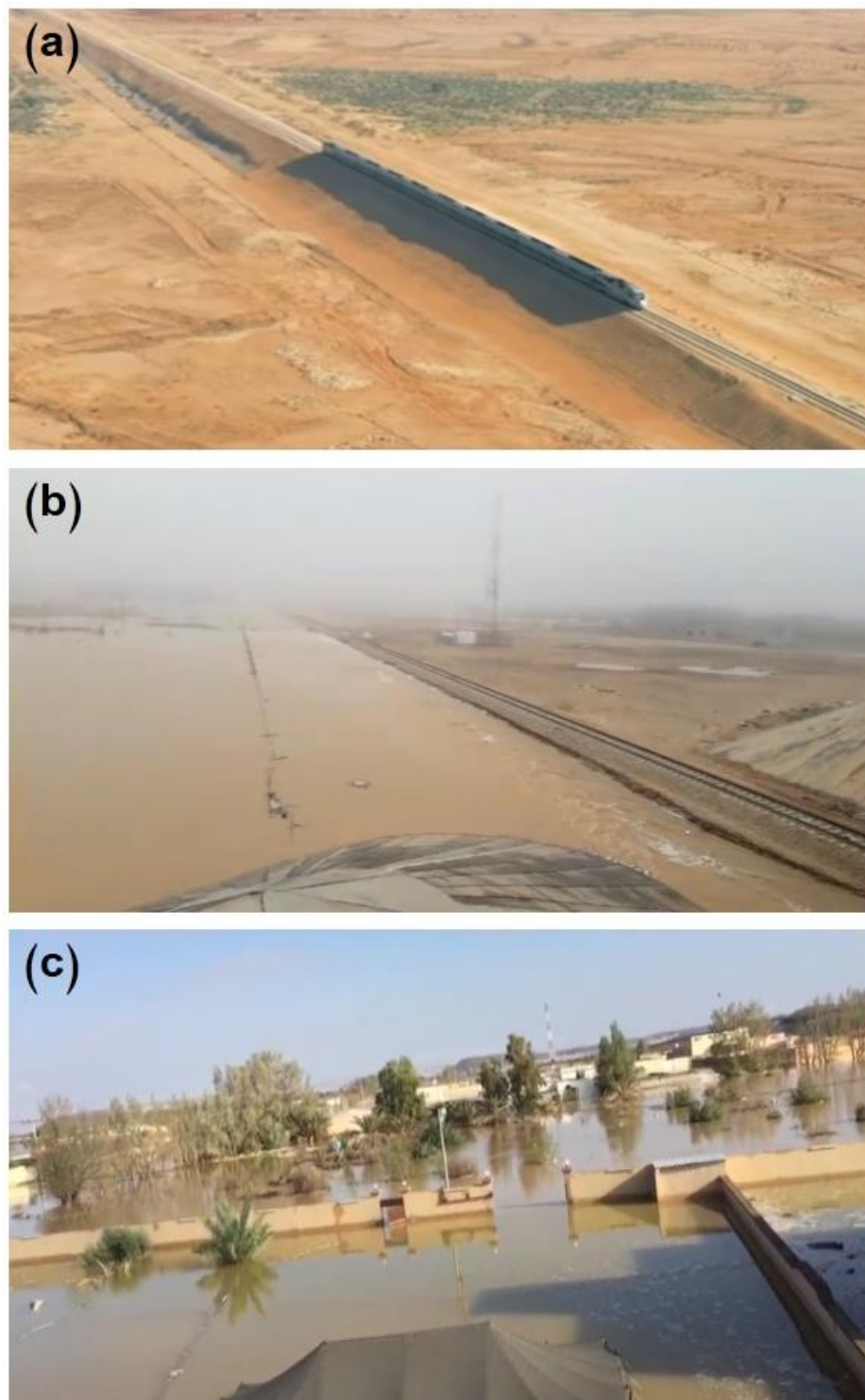
Figure 1. (a) Change in the natural appearance of land-use due to the presence of the Al-Shamal train pathway, which impedes the natural wadi runoff; (b) detaining of Wadi Bayer floodwater in front of the Al-Shamal train pathway on 10 November 2018; and (c) flooding of Bayer village due to the detaining of floodwater in front of the Al-Shamal train pathway on 10 November 2018.
