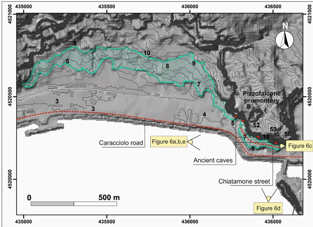
**Figure 5.** High-resolution DTM of the study area (1 × 1 m) with the first order paleo-shore platform highlighted with inclined green lines, contour lines in grey, elevation spots in black, and the roads described in the main text in dashed red.
