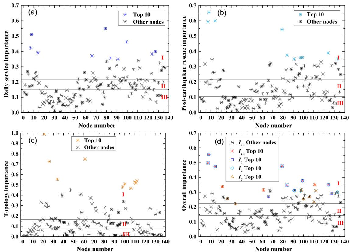
**Figure 11.** Importance values and classification of nodes obtained by TOPSIS. (a) Daily service ( $I_1$ ). (b) Post-earthquake rescue service ( $I_2$ ). (c) Network topology influence ( $I_3$ ). (d) Overall importance of all indices.
