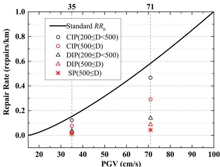
Figure 8. Pipeline repair rates evaluated by the fragility model of JWWA.
