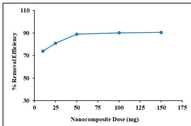
Figure 10. Effect of adsorbent doses on MB removal efficiency.
