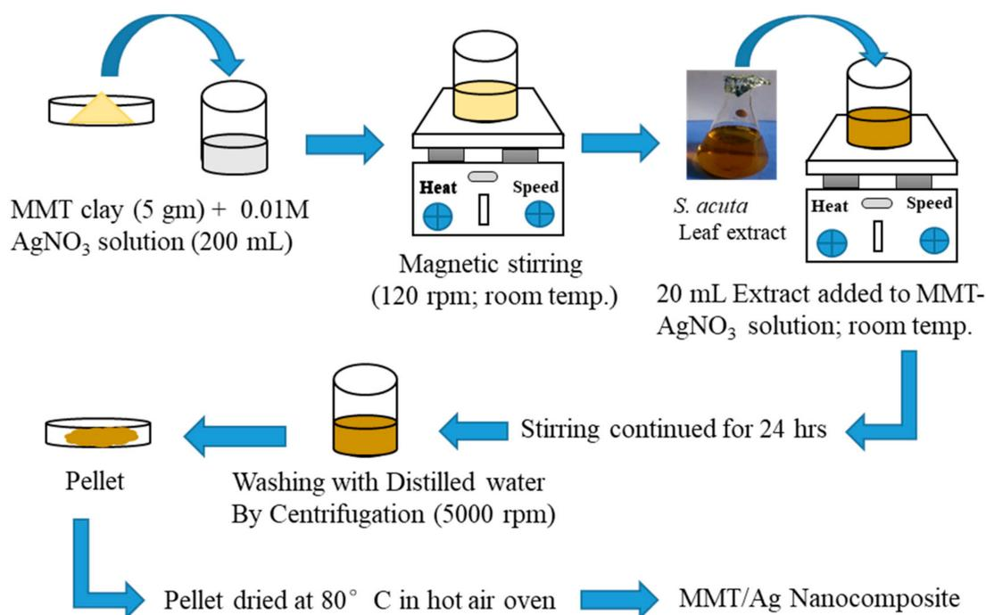
**Figure 3.** Synthesis process of MMT/Ag nanocomposite.
