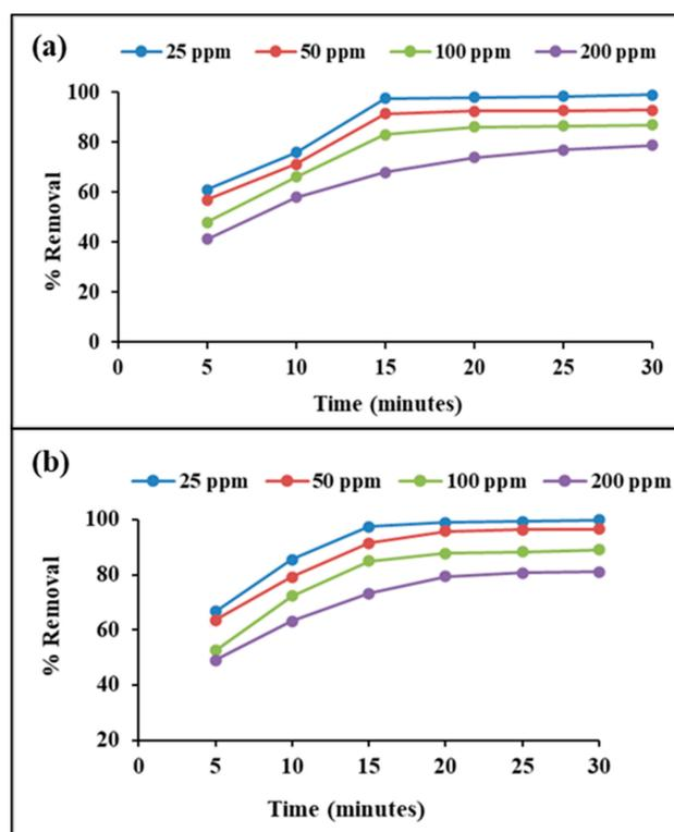
Figure 8. Removal percentage of MB using (a) MMT clay and (b) MMT/Ag nanocomposite.
