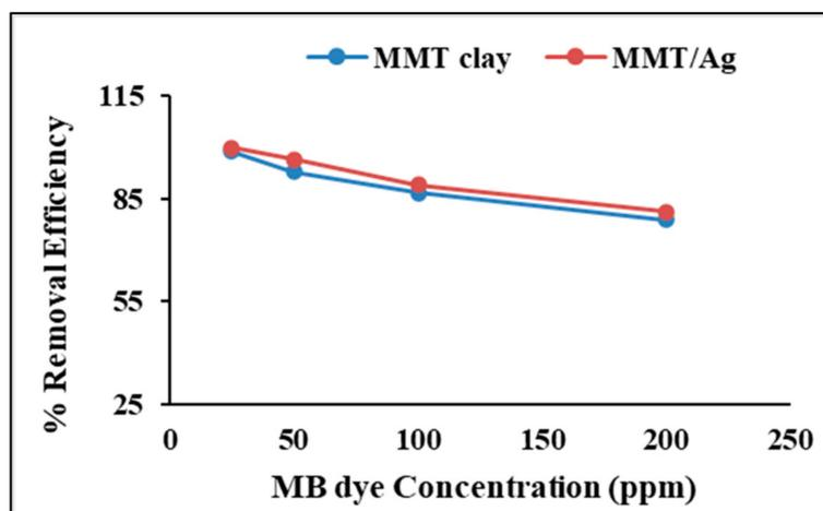
Figure 9. Effect of initial MB concentration on adsorption by raw MMT clay and MMT/Ag nanocomposite.
