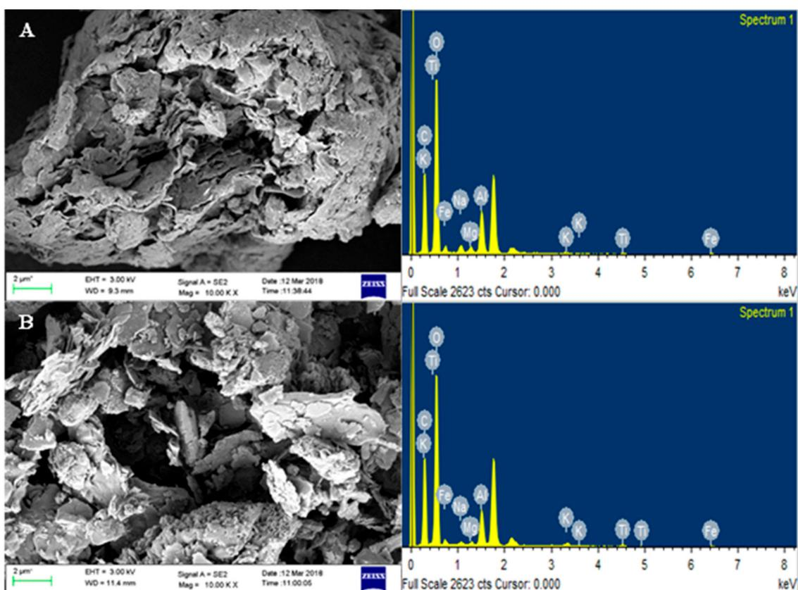
**Figure 7.** FESEM images and EDX spectrum of (A) MMT clay and (B) MMT/Ag nanocomposite.
