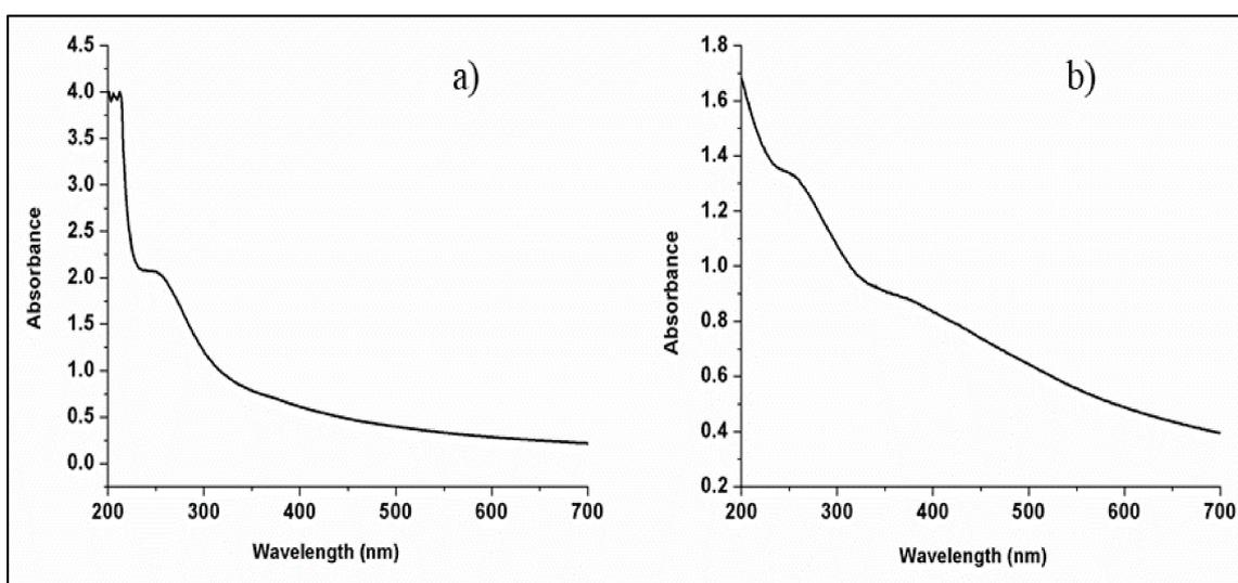
**Figure 5.** UV-Vis spectra: (a) MMT clay and (b) MMT/Ag nanocomposite.
