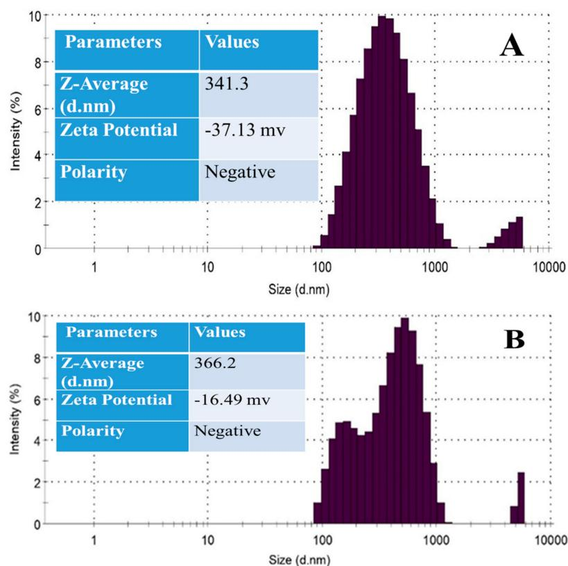
**Figure 4.** PSA graph of (A) MMT clay and (B) MMT/Ag nanocomposite.
