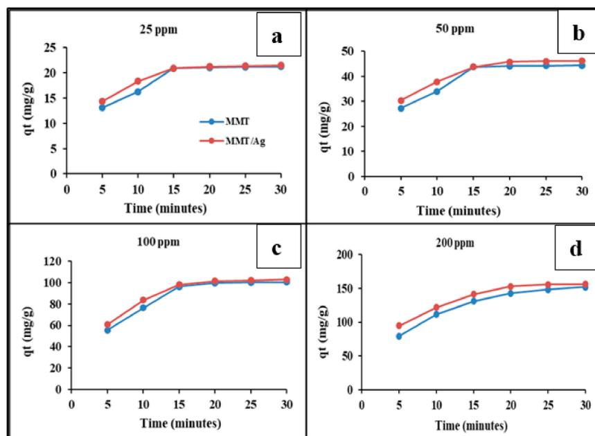
**Figure 11.** Effect of the contact time on adsorption capacity of raw MMT clay and MMT/Ag nanocomposite (a) 25 ppm, (b) 50 ppm (c) 100 ppm and (d) 200 ppm of dyes.
