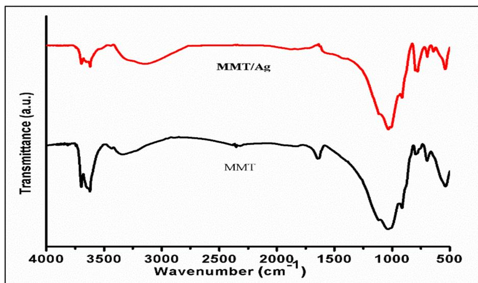
Figure 6. FTIR spectra of MMT and MMT/Ag nanocomposite.
