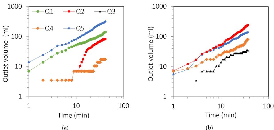
**Figure 5.** Outlet volume (mL) vs. time (min) at different test sections for (a) Fracture-2 with a fracture inclination of  $45^\circ$ ; (b) Fracture-4 with a fracture inclination of  $45^\circ$ .
