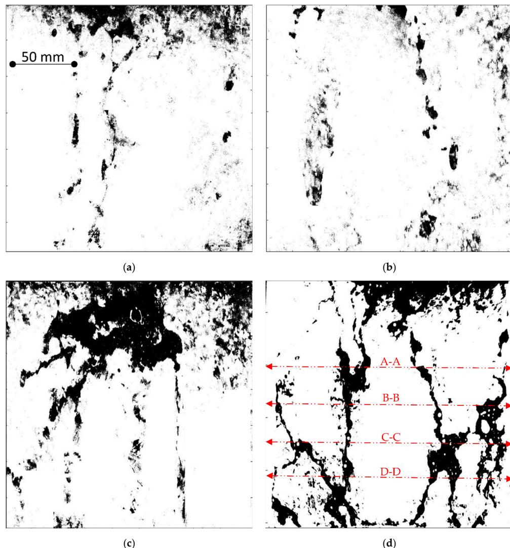
**Figure 9.** Preferential flow paths in the fractures with different fractal dimensions and mismatch lengths for inclination angle of  $\alpha = 45^\circ$ , 10 min after the start of the infiltration processes in the fracture: (a) Fracture-1; (b) Fracture-2; (c) Fracture-3; (d) Fracture-4.
