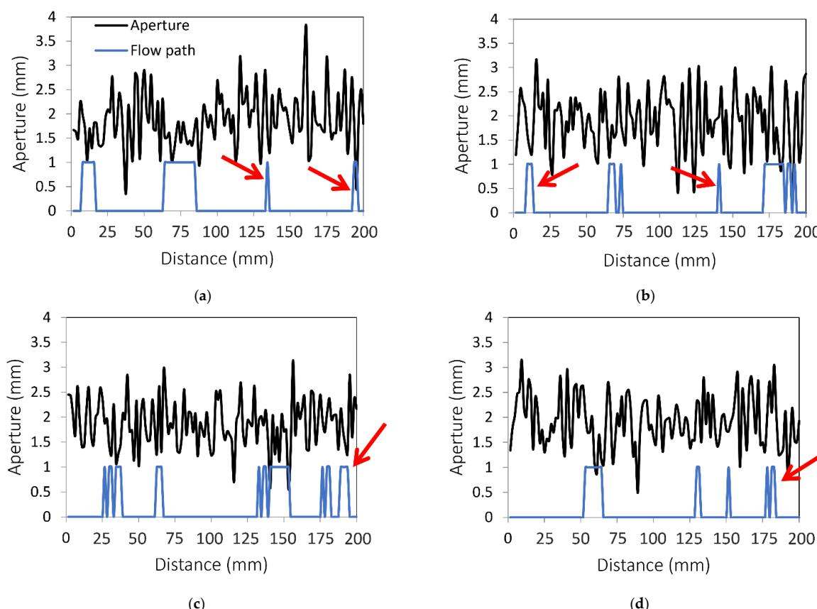
**Figure 10.** Flow paths along the aperture over cross sections: (a) A–A; (b) B–B; (c) C–C; (d) D–D. Red arrows indicate the flow paths with the maximum flow rate.
