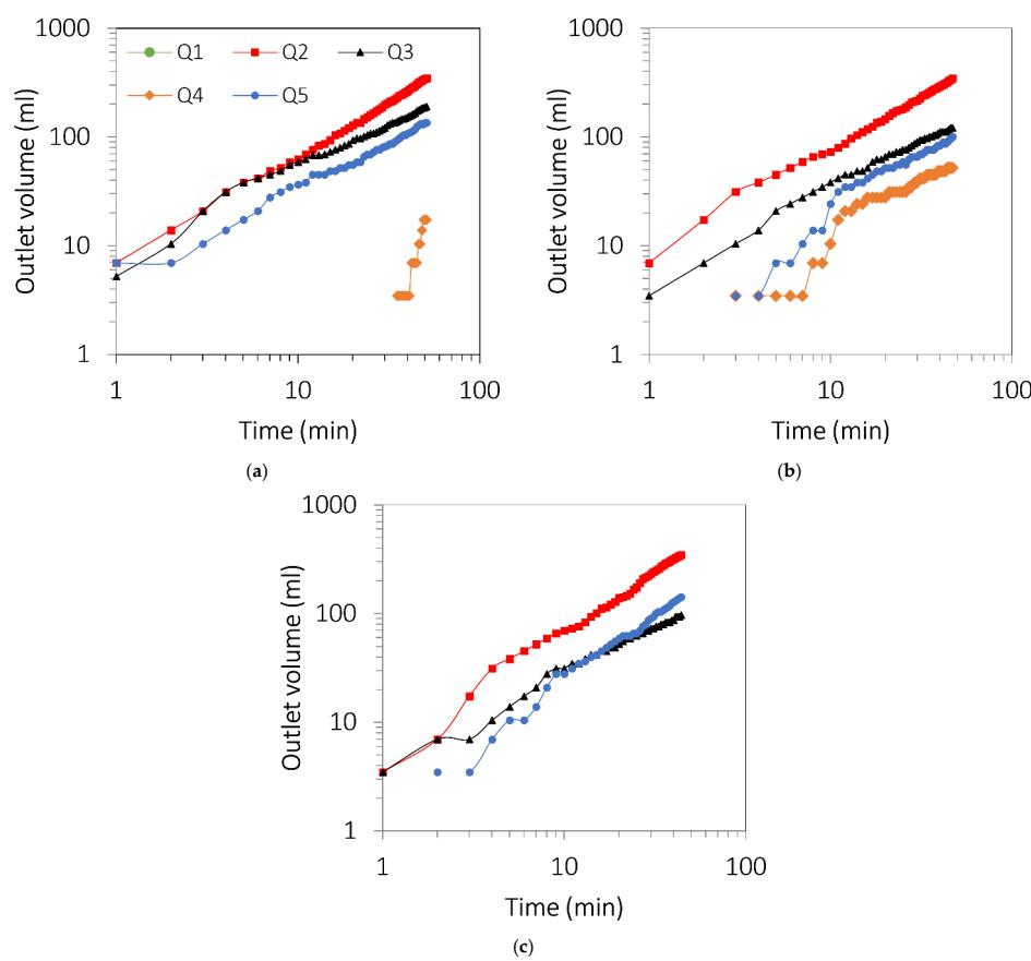
**Figure 4.** Outlet volume (mL) vs. time (min) at different test sections for Fracture-1, with an inclination of (a)  $45^\circ$ ; (b)  $55^\circ$ ; (c)  $65^\circ$ .
