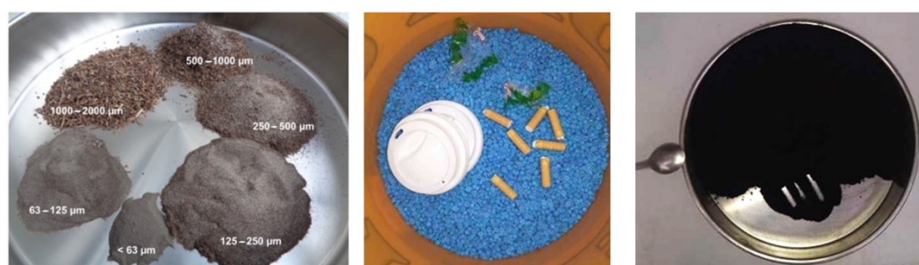
Figure 2. Test substances from left to right: real street dust, defined substances and tyre powder.
