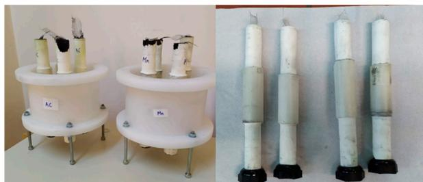
**Figure 2.** Ceramic electrodes produced.
