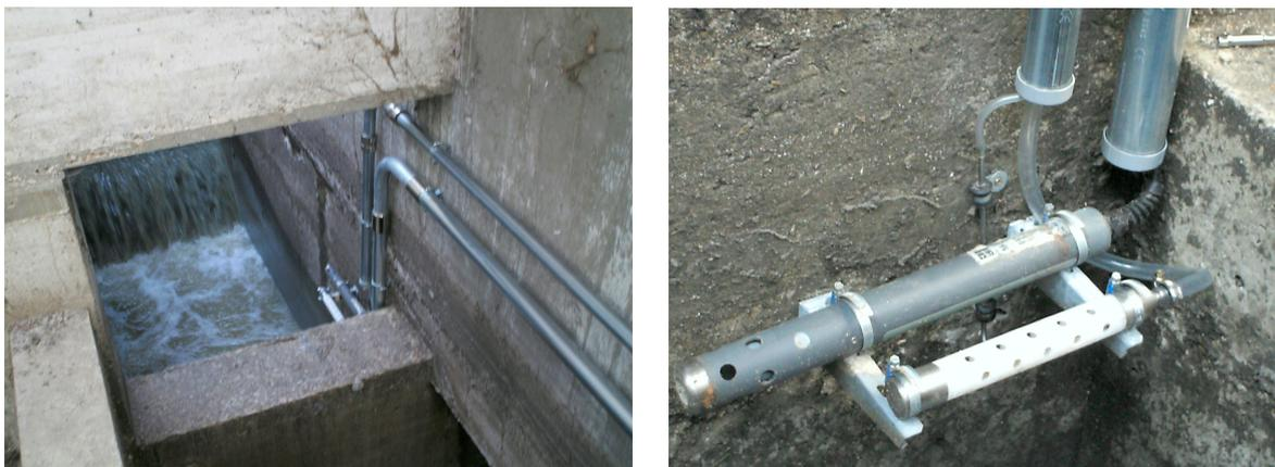
**Figure 2.** Positioning and detail of the monitoring equipment: bubble level meter and sampling probe.
