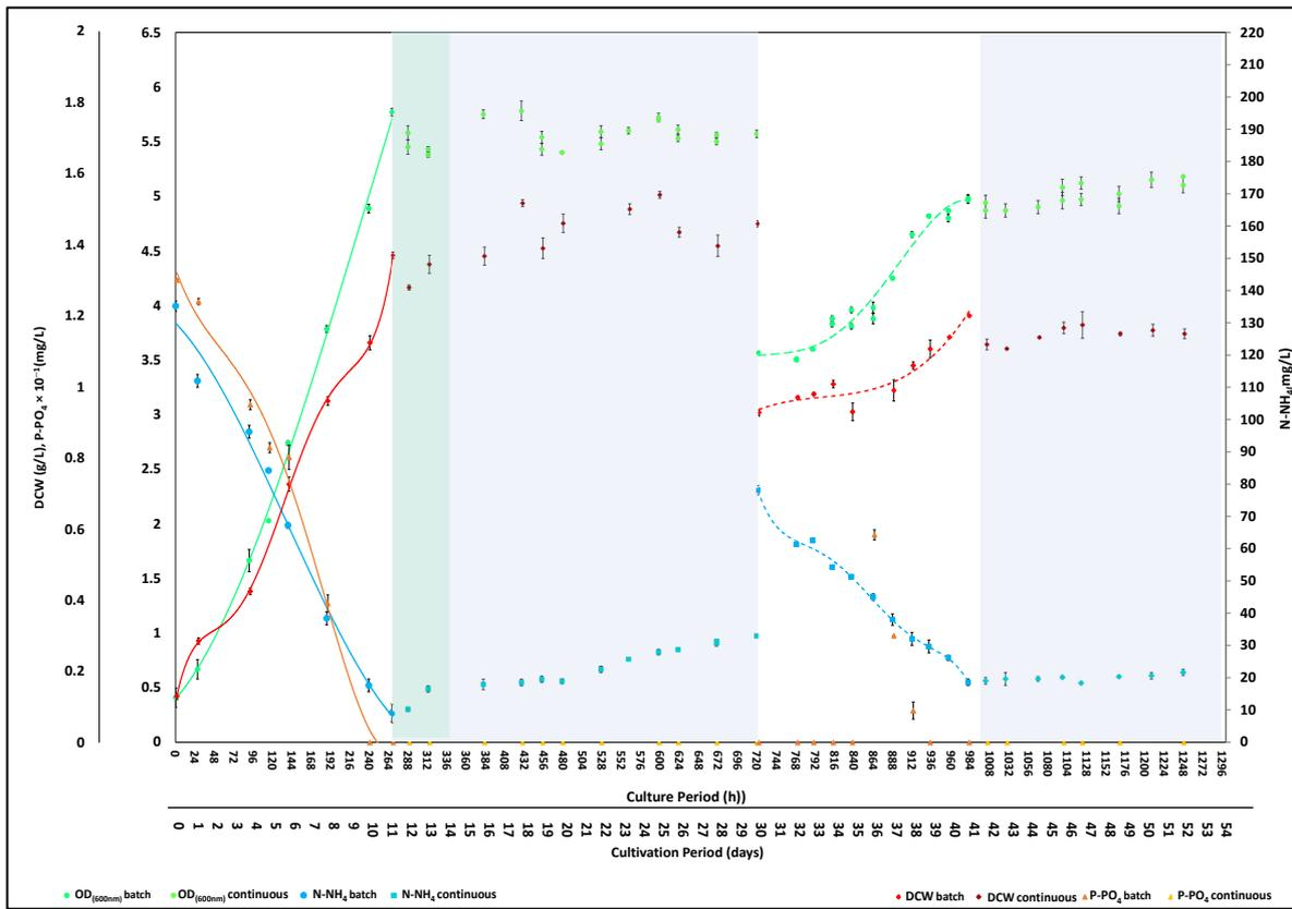
Figure 10. Time profile of the microalgae biomass, N-NH<sub>4</sub>, and P-PO<sub>4</sub> concentrations during the continuous operation of the ATPBR.
