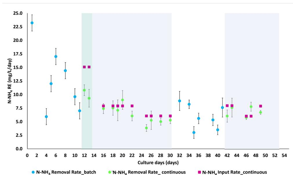
**Figure 12.** Ammonia nitrogen feeding and recovery rate by microalgae during the long-term operation of the ATPBR in continuous mode of operation.
