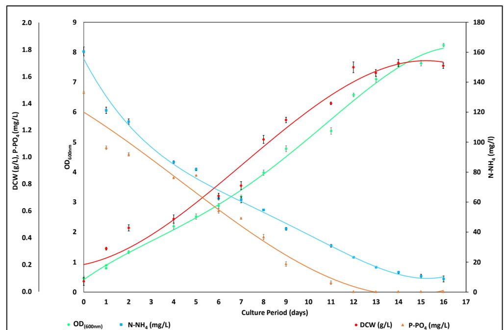
**Figure 3.** Microalgae growth and nutrients consumption as a function of cultivation time under *C. sorokiniana* cultivation in 5% ADE\_1.
