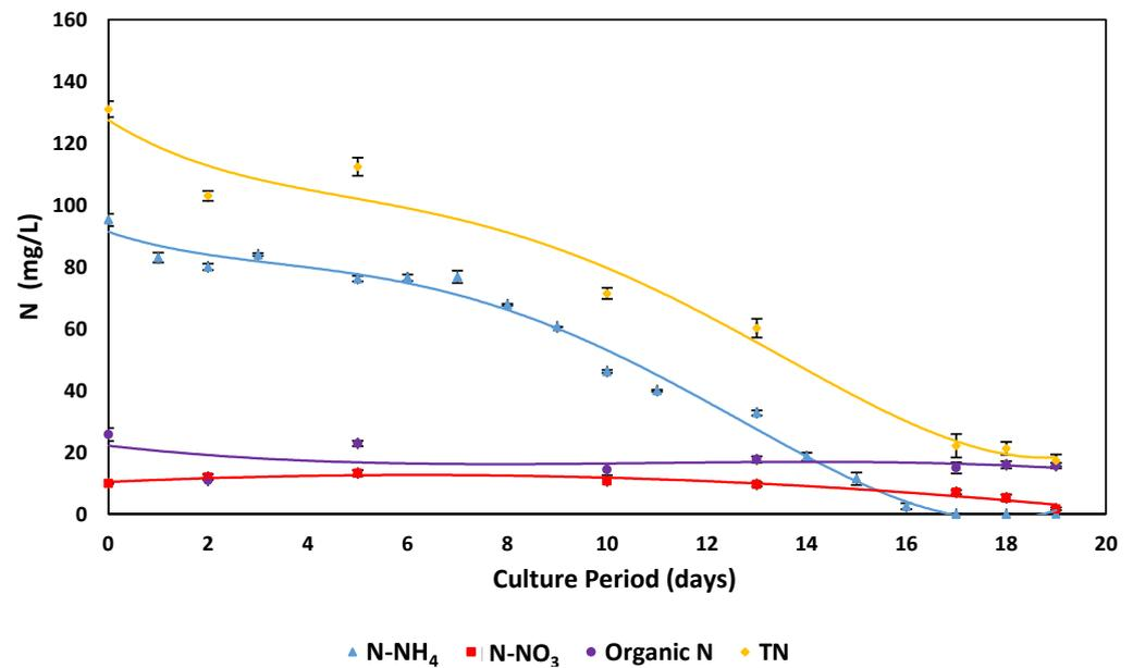
**Figure 4.** Consumption of the different nitrogen forms by *C. sorokiniana*, as a function of cultivation time using 3% ADE\_1.
