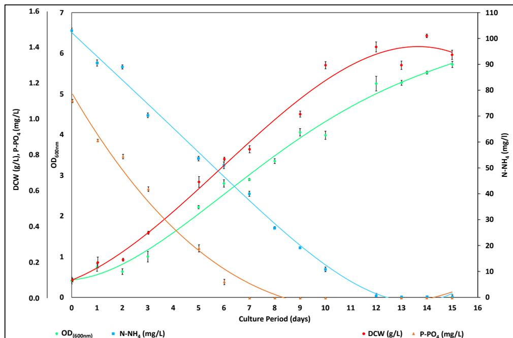
**Figure 6.** Microalgae growth and nutrients consumption as a function of cultivation time, under *C. sorokiniana* cultivation in 5% ADE\_2.
