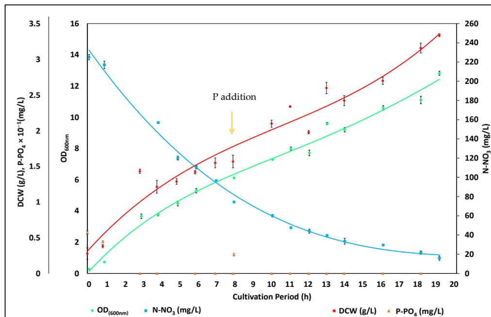
**Figure 1.** Microalgae growth and nutrients consumption as a function of time under *C. sorokiniana* cultivation in BG-11.
