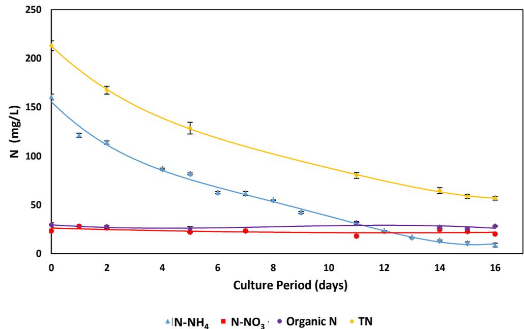
**Figure 5.** Consumption of the different nitrogen forms by *C. sorokiniana*, as a function of cultivation time using 5% ADE\_1.
