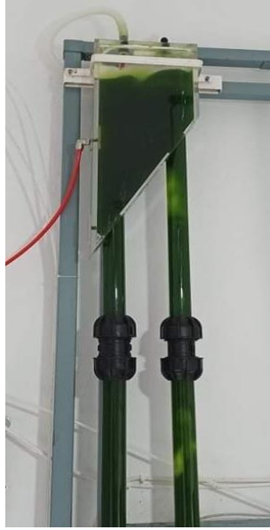
Figure S2: Airlift tubular photobioreactor: solar receiver part (a-b), degasser (c)
