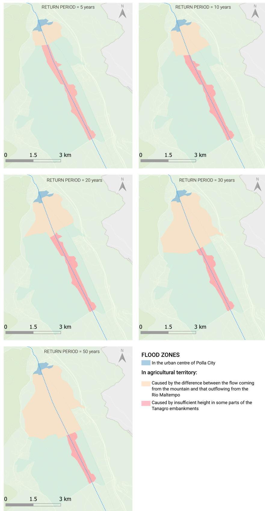
**Figure 6.** Cartographic delimitation of the flood-prone areas for flood events with different return periods—Vallo di Diano.
