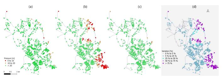
**Figure 6.** Spatial distribution of minimum pressures in nodes for year 20, at the peak-hour consumption (2 h): (a) Reference scenario; (b) Scenario 1 (demand increase and low rehabilitation rate); (c) Scenario 2 (demand decrease and adequate rehabilitation rate); and (d) Relative variation from Scenario 1 and Scenario 2 with respect to the reference scenario.
