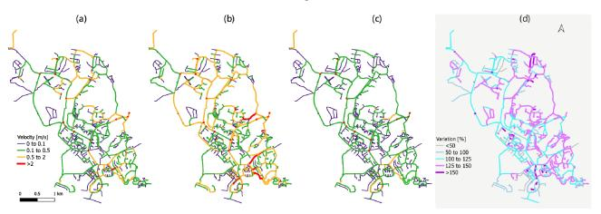
**Figure 7.** Spatial distribution of maximum velocities in pipes for year 20 at the peak-hour consumption (2 h): (a) Reference scenario; (b) Scenario 1 (demand increase and low rehabilitation rate); (c) Scenario 2 (demand decrease and adequate rehabilitation rate); and (d) Relative variation from Scenario 1 and Scenario 2 with respect to the reference scenario.
