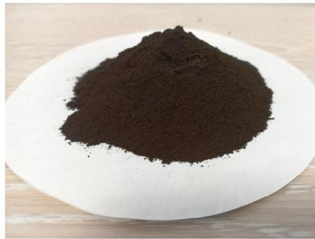
**Figure 2.** The sample of the obtained iron-containing sediment after ferritization of the etching solution.
