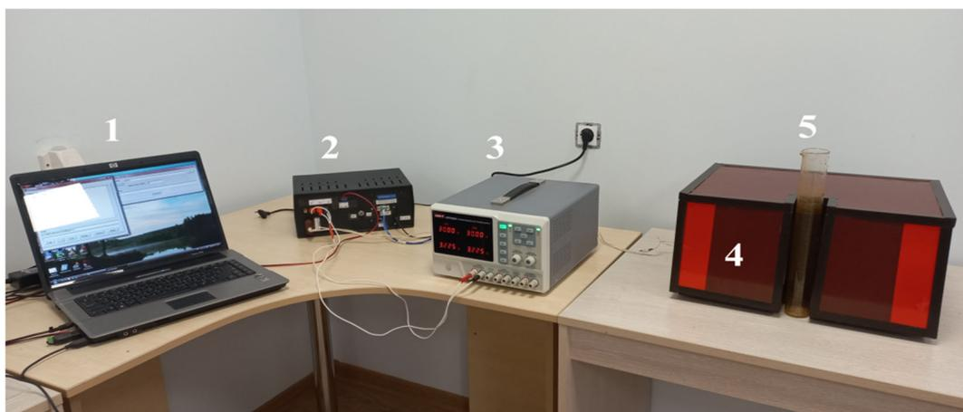
**Figure 1.** Laboratory ferritization installation with activation of the reaction mixture with alternating magnetic fields: 1—computer; 2—electronic block-case; 3—power supply; 4—electromagnetic coil with a steel core; 5—reactor with study solution.
