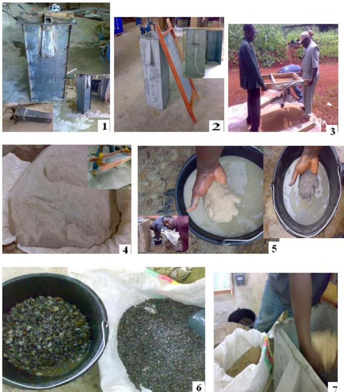
Figure 2. Plates showing the steps used in the construction, media preparation, and operation of the concrete intermittent bio-sand filters.
