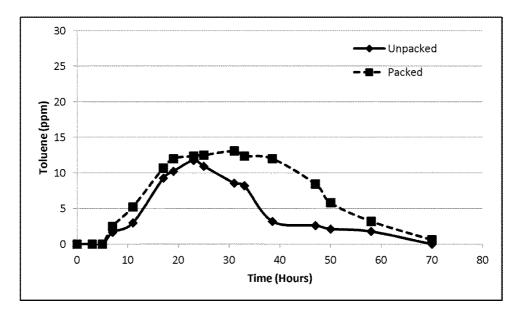
Figure 3. Toluene degradation results for unpacked system.
