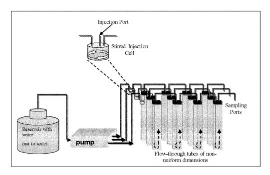
Figure 1. Schematic of flow-through microcosms.
