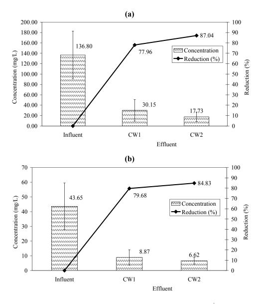
Figure 5. Average removal for (a) TKN ( $\pm$ SD) and (b) TP ( $\pm$ SD).
