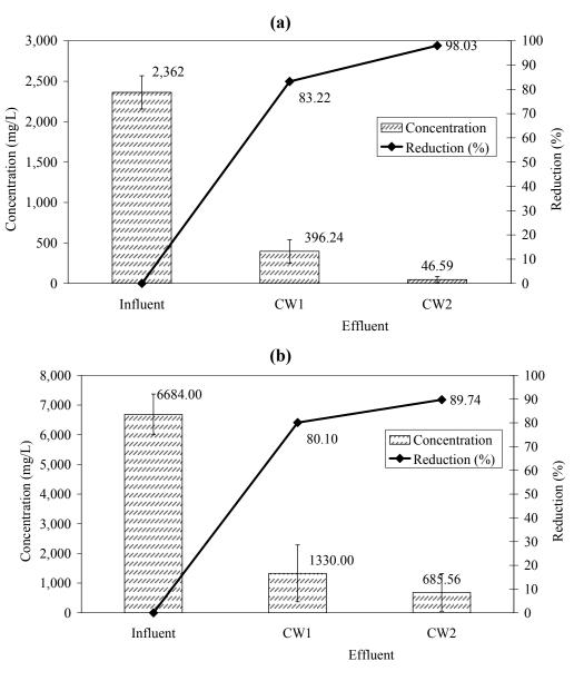
**Figure 4.** Average removal for (a) TSS ( $\pm$ SD); (b) COD ( $\pm$ SD); and (c) total phenols ( $\pm$ SD).
