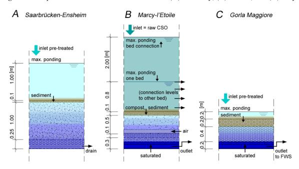
Figure 2. Simplified cross-sections of CSO-CWs in (A) Germany, (B) France; and (C) Italy.
