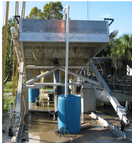
Figure 4. PVC piping system used to create sheet flow over simulated roadway.
