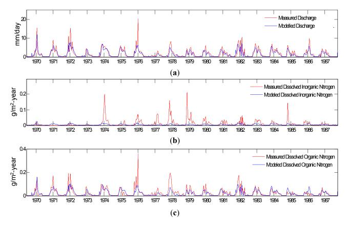
**Figure 5.** Measured *versus* model time series for stream water discharge (**a**), dissolved inorganic nitrogen (**b**) and dissolved organic nitrogen (**c**). Nash-Sutcliffe efficiencies for discharge is 0.71, for DON is 0.53. For DIN the efficiency is -0.13, as discussed in the text, this is likely due to the clearcut that occurred in the watershed in the early 1970s. The model did not attempt to incorporate the effects of the management.
