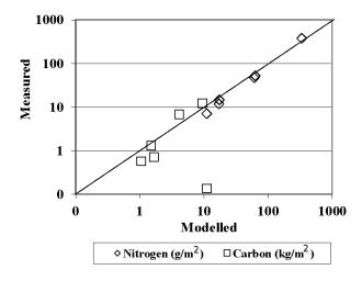
**Figure 3.** Measured *versus* modeled annual yearly storage of nitrogen and carbon. These data are also plotted in Figure 2. Each data point represents a different storage term, as outlined in Figure 2. A one to one line is included for reference.
