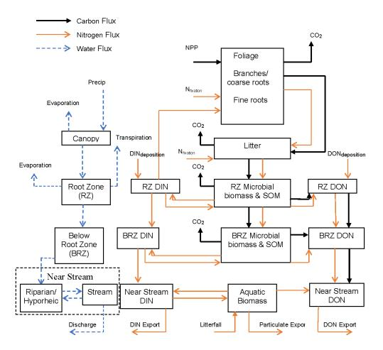
**Figure 1.** A flow chart outlining key model stocks and fluxes. Some minor flux terms have been left out of the figure to improve clarity. Note also that the litter input into aquatic biomass is derived directly from the stocks of foliage and branches/coarse wood.
